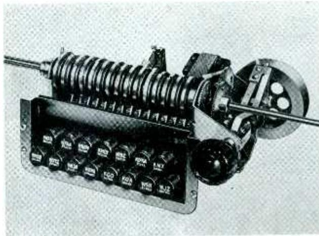
15 push buttons of Stewart Warner, eccentric discs stop shaft at station settings.
