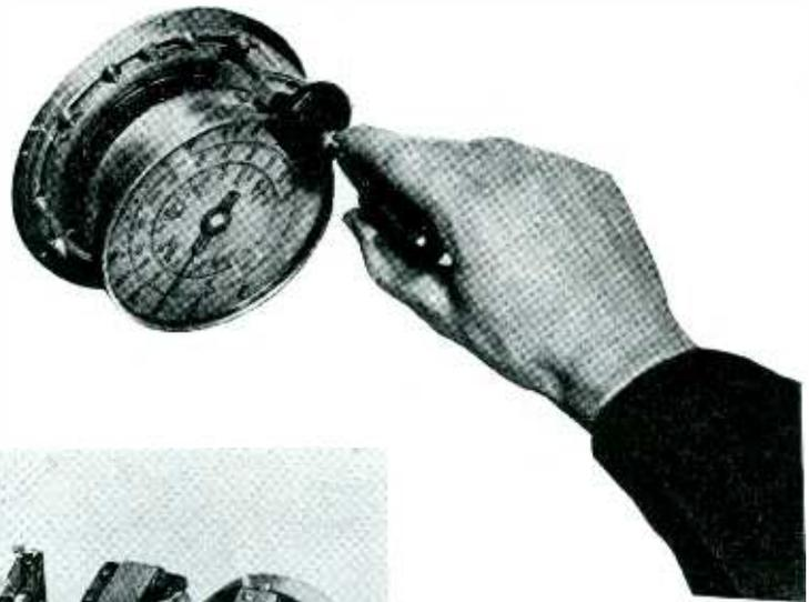
Setting Philco Cone-centric dial requires special tool, inserted through tuning knob.
