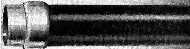
In IRC Type MP High Frequency Power Resistors, the "Metallized" element is applied solidly over a ceramic surface. Excellent characteristics at ultra-high frequencies of more than 75 mc result.
