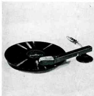
**PICKUP**—Model AT-12, a low priced pickup that is designed to approximate compensated microdyne performance for records up to 12 in. Smart, streamlined offset head, response to over 6000 cycles, new needle guide, new non-resonant arm, precision ball-bearings, 200-500 ohms or high impedance.
