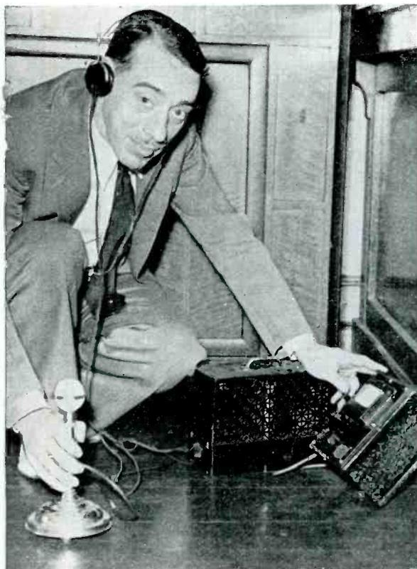
**FASCINATES PROSPECTS**—With the aid of an amplifier and output meter Stanley Almas checks noise levels
