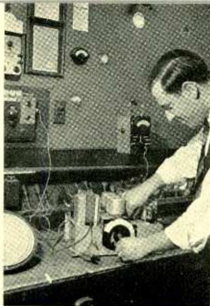
**"MONORAIL" OHMMETER** — Joseph Scotti; rides his volt-ohmmeter monorail style on two pulleys running on a tight wire across the bench, substitutes his signal generator for the oscillators in superhets with unknown i.f.'s
