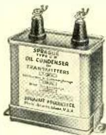
**CONDENSERS** — "Neutrol" rectangular transmitting condenser with flanges for mounting in any position combine oil-filled, oil-impregnated construction with rectangular sizes. Labeled with information concerning capacity, maximum d.c. working voltage and maximum surge voltage. Oil has a flash-point of 500 degrees F. *Radio and Television Retailing, June,*
