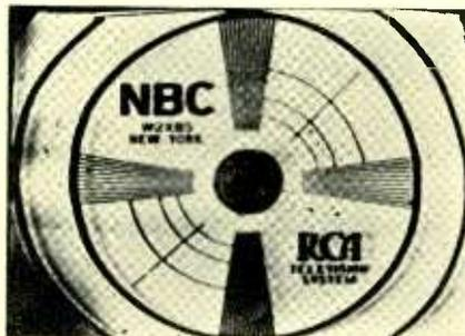
FIG. 3—Only a single ghost appears in the above pattern. The ghost signal in this case was probably a reflection from the Chrysler building. The intensity of the ghost is sufficiently lower than the direct image so as not to be troublesome when viewing pictures in motion. The reduction in images was achieved by rotating the antenna so the broadside faced the Empire State Building
