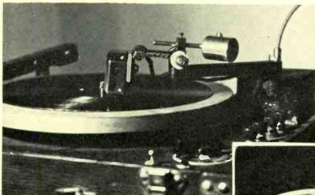
**ADJUST CUTTING HEAD ANGLE**—To avoid “chatter”, “tear”, cuts either too deep or too shallow, the stylus should be at the correct angle with respect to the blank. Two degrees is generally right for acetate
