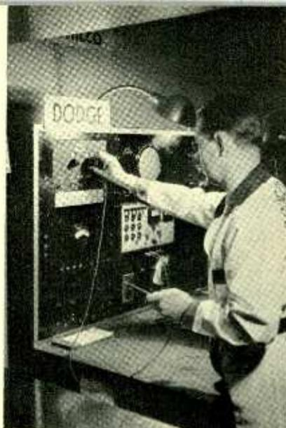
**ALIGNMENT BY REMOTE CONTROL** — Harry Dodge trims up receivers in police cars at his curb by hooking an antenna to his signal generator inside the shop
