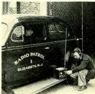
**OSCILLATOR** — Portable oscillator makes it possible to check high frequency signals without removing receiver from radio patrol cars. Can be used for zero-beat frequency check on transmitter. Jack provided on oscillator panel for insertion of earphones. Can generate fundamental signals ranging from 22 to 150 mc. at an accuracy of 1 per cent, is adaptable to use in television, aviation, and other fields employing ultra high frequencies. *Radio and Television Retailing, June, 1939.*
