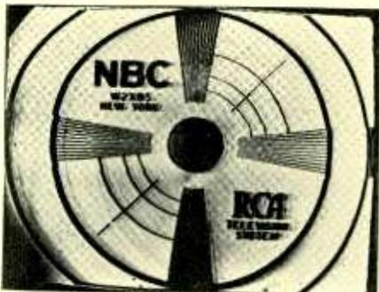
FIG. 2—An improved image with several smaller ghosts. Note particularly the double and triple images on the letters RCA and to the right of the bottom vertical wedge. No tuning adjustments were made in the receiver between this pattern and that of Fig. 1 or 3. A doublet receiving antenna was used
