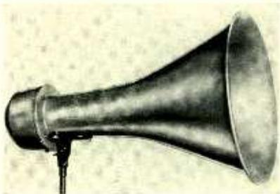
**CONE PROJECTOR**—"Super-Power" projector for 8 in. speakers includes true exponential design which results in an adequate loading of the cone diaphragm for added efficiency and power handling ability. Suitable for use for all out-door P.A. applications, and industrial uses. Bell diameter 24 in., total length 36 in. Finish is battleship gray weatherproof lacquer. Model G-8, List \$22.00. *Radio and Television Retailing, June, 1939.*
