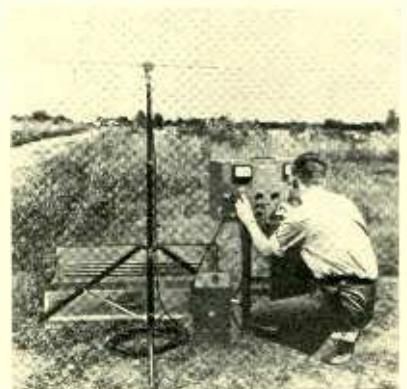
**TESTER**—A new portable measuring instrument for surveying the service range of television and other stations operating in the ultra high frequency spectrum of from 20 to 125 mc., provides accurate indications of the strength of very short wavelength signals, enables records to be made automatically with suitable attachments, provides data on the amount of noise which might interfere with television pictures. *Radio and Television Retailing, June, 1939.*
