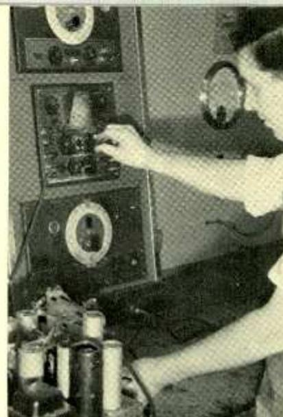
**BRUTE FORCE PLUS BRAINS**—W. C. Siegrist tags intermittents by boosting line voltage with an auto-transformer, watching for part failures on the screen of his oscillograph
