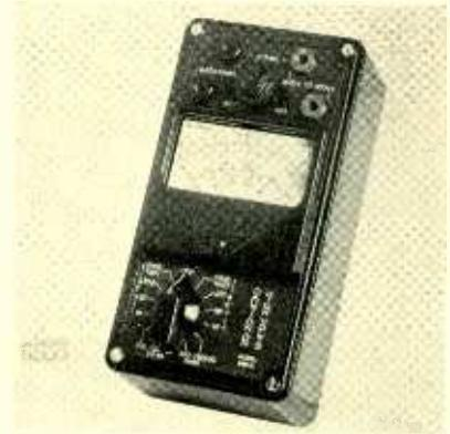
**TESTER**—Model 666-H a.c.-d.c. pocket volt-ohm-milliammeter will handle voltages to 5000 volts without external multipliers. Checks high voltages and circuits of transmitters and receivers. Selector switches for all readings. A.c.-d.c. voltage at 1000 ohms per volt—0-10-50-250-1000-5000; d.c. milliamperes—0-10-100-500; resistance 0-300 ohms; 0-250,000 ohms, with provision for higher measurements by using external batteries. List \$21.75. *Radio and Television Retailing, June, 1939.*
