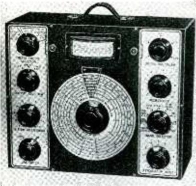
**MICROVOLTER**—Crystal controlled signal generator with self contained vacuum tube voltmeter and power level meter. Provides signals from 100 kc. to 15,000 kc. at 100 kc. points; also 1000 kc. to 100 mc. at 1000 kc. points. Accuracy better than .01 percent. R.f. output from 1/2 to 100,000 microvolts. Seven radio frequency ranges calibrated directly from 100 kc. to 60 mc. Hickok Electrical Instrument Co., 10514 Dupont Ave., Cleveland, Ohio.
