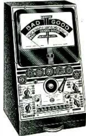
**GIANT TESTER**—Model 325 tube tester with large rectangular 9 inch meter indirectly illuminated by two 6 volt bulbs. Complete range of filament voltages from 1.5 to 120 volts. Tests local, single-end, bantam, midjets, ballasts, gaseous rectifiers and Christmas tree bulbs. Individual toggles test each element separately. Line adjustment, short and leakage tests, headphone jack for noise tests. Simpson Elec. Co., 5216 Kinzie St., Chicago, Ill.
