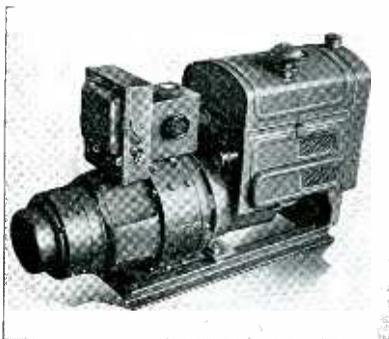
**POWER PLANT**—A 5 k.w. gas electric power plant designed for heavy duty. Engine completely enclosed in sheet metal housing to protect it from dirt, dust and rain. Uses 4 pole generator rotating at 1800 r.p.m. Complete with rheostat, voltmeter and switchbox. Filter and shielding available for radio operation. Pioneer Gen-E-Motor Corp., 466 W. Superior St., Chicago, Ill.
