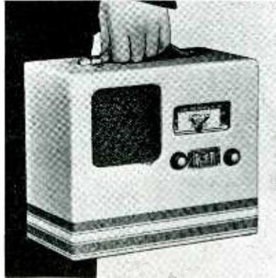
**PORTABLE**—Model 802 operates on self-contained batteries or electric current; 250 to 350 hours operation on one set of batteries; 5 tubes and built-in antenna; band coverage from 540 to 1750 kc., provides a separate compartment for electric cord when not in use; measures 12 3/8 wide, 10 3/4 high, 6 1/2 inches deep. Covering is airplane luggage cloth, with heavy-gauge sewn leather handle; list \$24.95.
