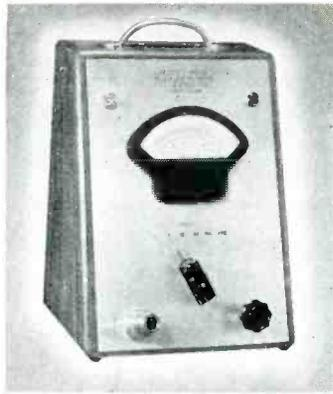
V. T. VOLTMETER—Model VG-6 full-wave square-law type infinite impedance vacuum tube voltmeter. Readings not affected by harmonics; frequency error is 3 per cent between 40 cycle and 56 mc.; furnished with coaxial test cable; voltage range from 2 to 600 volts in 6 steps; a.c. or d.c. scales selected by toggle switch. Televiso Co., 337-345 N. Crawford Ave., Chicago, Ill.
