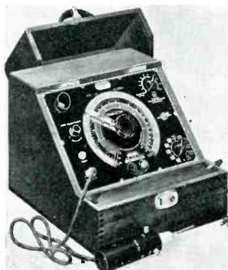
EXAM-ETER—New circuit and component analyzer. Serves as output indicator, dual range peak-voltmeter; r.f. alignment indicator; capacitance bridge; resistance bridge; power factor indicator; leakage indicator; and continuity checker. Solar Mfg. Co., Bayonne, N. J.
