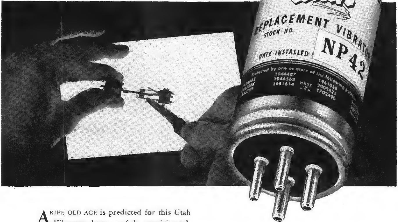
**A** RIPE OLD AGE is predicted for this Utah Vibrator—because of the precision adjustment of the contact points. This delicate operation, performed by the hands of skilled and experienced technicians, is responsible not only for the long life of Utah Vibrators, but for their correct electrical balance, current output, and freedom from noise.
