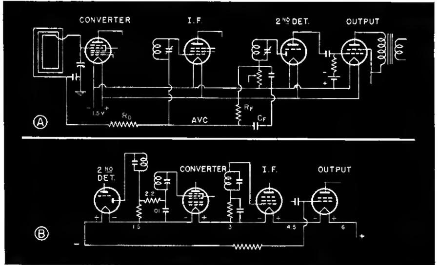
Fig. 1—Typical circuit of portable with parallel filament arrangement (A) showing common type of AVC distribution. Diagram (B) is the typical series filament connection with AVC network.
