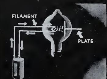
16 To show how a tube operates, this drawing illustrates an electronic circuit, with one battery heating the filament so that it can throw off the free electrons.
