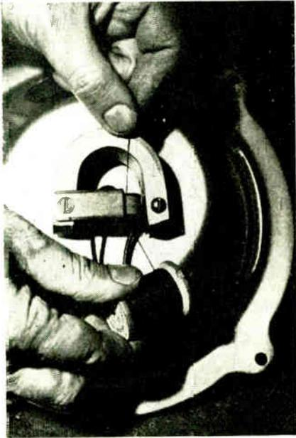
▲ When the armature of a magnetic speaker does not vibrate freely, this may be due to dust or rust between armature and pole pieces. A strong thread may be inserted as shown, and used to clean out the foreign matter.
