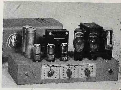
$\pm 1\frac{1}{2}$  db. Negative feedback and r-c coupling is used. A choice of high or low impedance input is optional, while the output impedances are 4, 8, 250 and 500 ohms. Mark Simpson Mfg. Co., 186 W. 4th St., New York 14, N. Y.—RADIO & Television RETAILING
