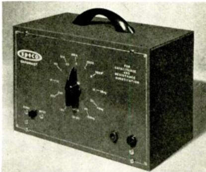
capacity values, from .001 to 40 mf, are selected by a multitap switch. Special Products Co., 9115 Brookville Rd., Silver Springs, Md.—RADIO & Television RETAILING
