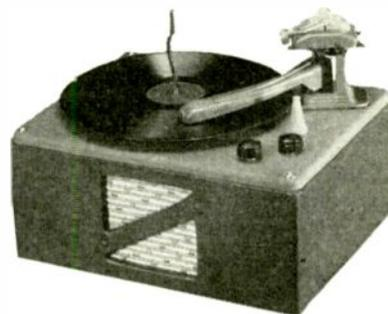
Record changer with Crescent Model No. 100, completely assembled with amplifier, ready to play. Cabinet of brown leatherette with 3/8" seasoned pine, rubber bumpers on base. Cabinet dimensions: 16" long, 12 3/4" wide, 6 1/2" high; height with changer 12". AC amplifier with heavy duty power transformer complete with tubes 6V6, 6C5, and 6X5, tone and volume controls, cord and plug, separate AC line switch, 6" speaker. Well constructed, excellent tone
