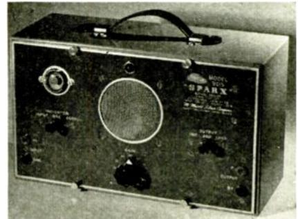
range is from 20 cycles to over 200 mcs. A 6E5 electron-ray tube indicates stage gain and voltages of dc and rf circuits. McMurdo Silver Co., 1240 Main St., Hartford 3, Conn.—RADIO & Television RETAILING
