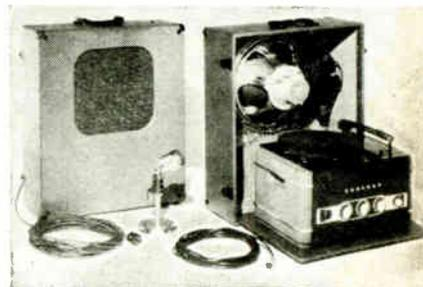
power. The two input channels can each handle microphones with a 120 db gain, and phonos with a 73 db gain. Besides the two channel gain controls, a bass-treble control, an off-on switch, and a pilot light appear on the front panel. 15 output impedances are supplied, ranging from 1.3 to 600 ohms. Hum level is 65 db below full signal, and frequency response is 50-10,000 cycles. Concord Radio Corp., 901 W. Jackson Blvd., Chicago 7, Ill.—RADIO & Television RETAILING
