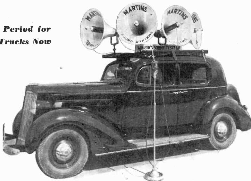
Sound dealer Max Martin of Ottawa, Canada, gets as much publicity as the candidate. A portable generator lights 100 W reflector bowl lamps mounted in the white-painted DR-72 Atlas trumpets.
