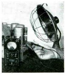
Applying radiant heat to "force" troubles.
