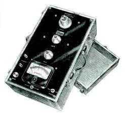
has 3 scales of 5, 10 and 20 kilovolts with a sensitivity of 10,000 ohms per volt. Shall-cross Míg. Co., Collingdale, Pa.—RADIO & Television RETAILING
