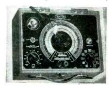
Solar Model CBB Capacitor Analyzer
