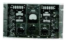
Model A-322C Limiter Amplifier compensates for volume variations resulting from changes in the speaker's position with respect to the mike, preventing blasting and loudspeaker overloads and allowing the use of a higher sensitivity in the PA system without feedback. A gain of 68 db with a response from 20 to 20,000 cycles is available, with a 5W output and 600 ohm input and output load impedances. Altec Service Corp., 250 W. 57th St., N. Y. 19, N. Y.—RADIO & Television RETAILING.
