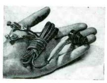
Ear-plug radio using no electricity, no batteries, no tubes. Tunes in stations when clips are attached to aerial and to ground. Can be used as telephone (up to 100 ft.) when two units are clipped to opposite ends of wires; talking and listening done through same rubber plug. \$2.98 retail. A. M. R. Corp., (representatives) Breslin Toy Mart, 1186 Broadway, New York 1, N. Y.—RADIO & Television RETAILING
