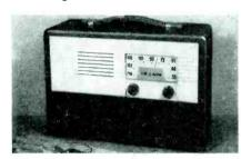
"Royal Troubadour" model portable 3way receiver, superhet with Alnico 5 PM speaker. Four miniature tubes plus metallic selenium rectifier, avc, die-cut antenna. Provision for external aerial. All-wood case bound in simulated leather. \$37.95. Air King Products Co., Inc., 1523 Sixty-third St., Brooklyn 19, N. Y.—RADIO & Television RETAILING
