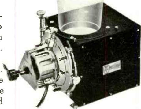
• The PROTELGRAM projection system consists of a specially developed 2½" projection tube, an optical box with focus and deflection coils, and a 25 kv regulated power supply unit. Compactness and flexibility make possible large-picture television in average size radio-phonograph consoles, consolettes and table model television receivers.
