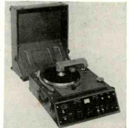
tive speed change; high fidelity amplifier for recordings and playing back; 16-inch pickup arm permits playbacks of 12-inch records and 16-inch transcriptions; 8-inch speaker; self-oiling system. Priced at \$319.95. Rek-O-Kut Co., Inc., 38-01 Queens Boulevard, New York, N. Y.—RADIO & TELEVISION RETAILING
