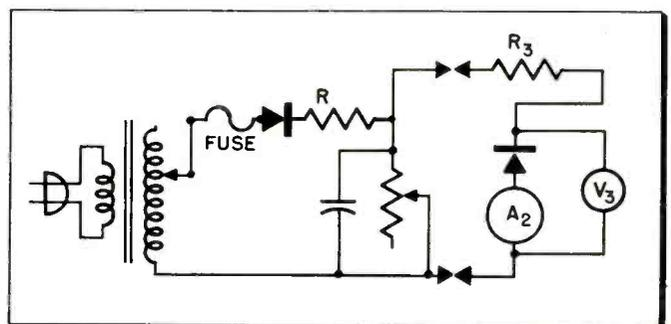
tions, or as close thereto as practical. It is possible to obtain a professional looking rectifier tester from test-instrument manufacturers. For the technician who enjoys the mechanics of basic electronic manipulations, the procedure is straight-forward and simple. The test set up is shown in Fig. 1. The values of the various parts used depend on the voltage and current ratings of the rectifier under test.
