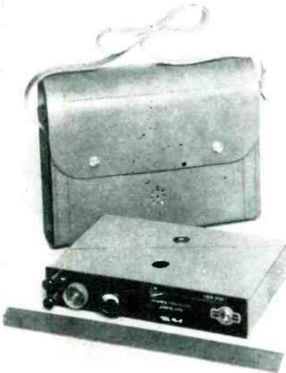
Self-contained battery-powered transistorized burglar alarm provides "watch while you sleep" protection for containers of currency and other valuables carried by couriers and messengers. A shrill and markedly audible signal is set off if an intruder enters the area of protection.
