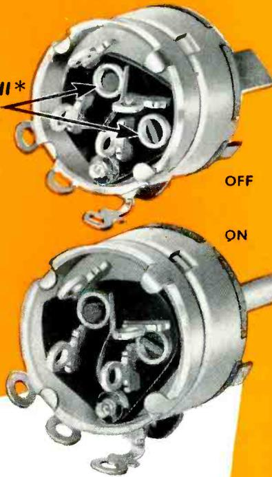
There's something new on Mally volume controls—a line switch with unique contact action. Make and break is accomplished by spring-snapped motion of "floating" rings of special Mally contact alloy. Rings rotate with each switch operation . . . presenting a constantly changing contact surface . . . providing these performance extras:
