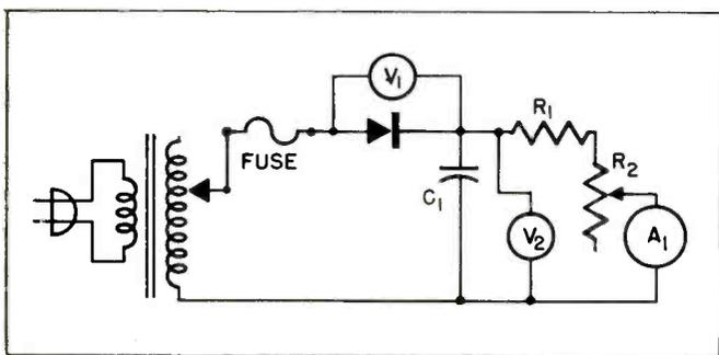
Fig. 2—Reverse current and reverse dynamic resistance is determined by connecting the rectifier back-to-back, to oppose the flow of current.
