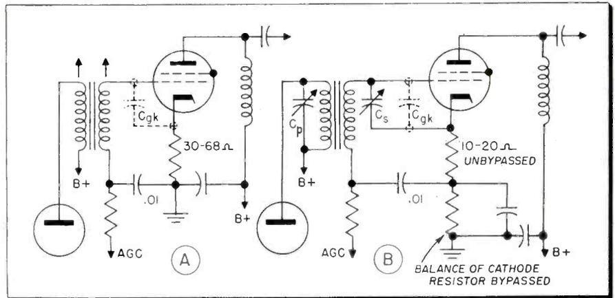
Fig. 3—Two ways of counteracting Miller Effect in TV i-f amplifier design are illustrated.
