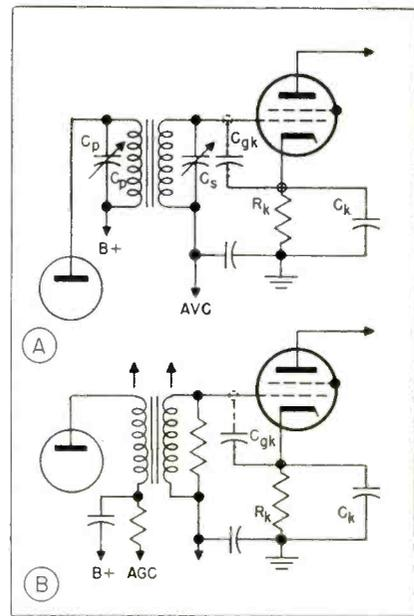
Fig. 2A—In AM i-f stage, large capacitors shunt i-f coils. B—Coils in TV i-f stage.
