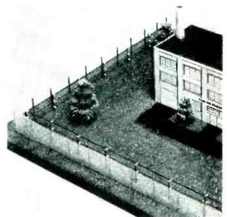
An entire industrial area can be secured from intruders with the electronic-fence alarm system. The inside, 3-wire fence shown, illustrates how an invisible electronic field is created around the perimeter of the area.
