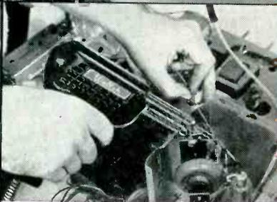
**4 SOLDERING BROKEN TERMINAL LEADS.** Weller Soldering Gun permits controlled application of heat. Solder is maintained at correct viscosity. This enables serviceman to produce rounded joints and prevent corona discharge in high-voltage compartment.
