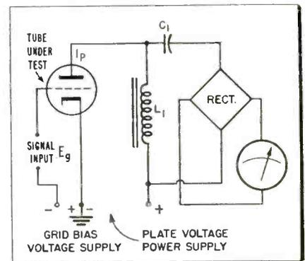
Fig. 2 Basic transconductance-test circuit.
