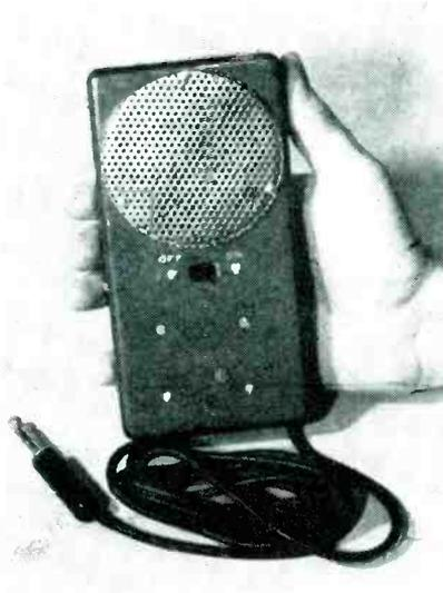
A small but powerful power amplifier and speaker utilizes 3 transistors. Its self-contained batteries will operate for over 700 hours. It is a practical and easily-handled accessory for any earphone-style tape or wire recorder, radio receiver, or amplifier. The unit is used in place of an earphone.
