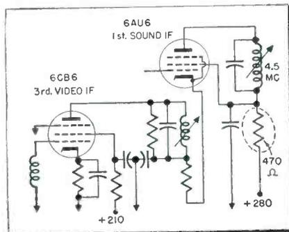
gone up in value. Hence the low voltage on the sound-IF plate, and in turn the low voltage on the 3rd-video-IF plate which caused the weak sound and video. Replacing the resistor returned the set to normal. *Frank A. Salerno, Long Island City, N.Y.*
