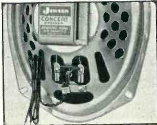
Three-way universal terminal-lead arrangement is especially convenient. Tip jacks fit Ford-Lincoln-Mercury rear seat pin terminals; twin lead for splicing to front seat plug cable; solder lugs for general use.
