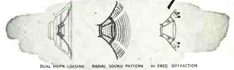
DUAL HORN LOADING RADIAL SOUND PATTERN HI FREQ. DIFFRACTION
