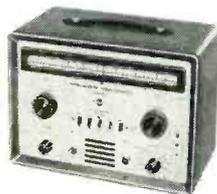
**WR-99A CRYSTAL CALIBRATED MARKER GENERATOR**—supplies fundamental-frequency rf carriers of crystal accuracy for use in aligning and trouble-shooting color and monochrome TV, FM, and other electronic equipment operating in the 19 to 260 Mc range. \$242.50\*
