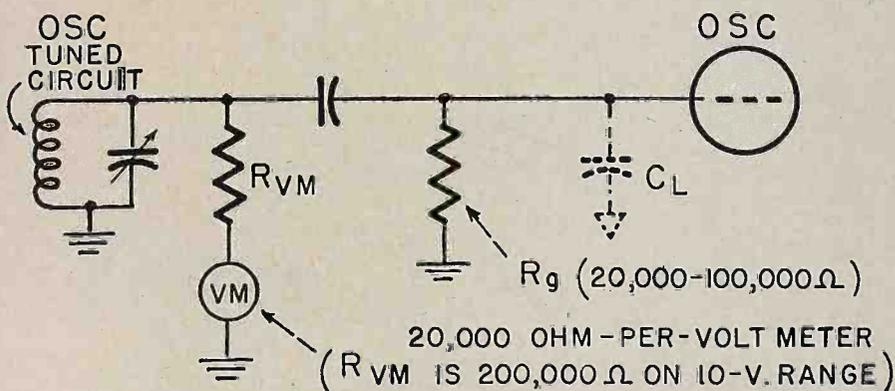
Fig. 2—Using a voltmeter with a relatively low input resistance will load down the tank circuit. If  $R_g$  is 100,000, and  $R_{vm}$ , the internal resistance of the meter, is 200,000, the effective value of  $R_g$  becomes about 67,000 ohms.
