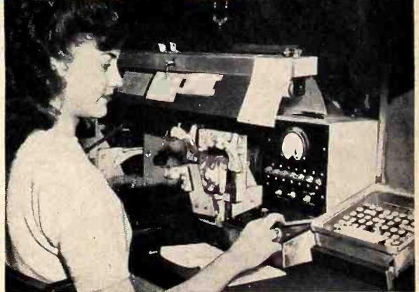
Test after test assure the uniform high quality of G-E tubes. Here G-E receiving tubes get a factory "short" test. Later comes an electrical-characteristics check; also tests for noise, microphonics, life, appearance, gas, air, and hum. G-E tubes perform better because they are better!
