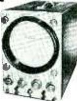
Uses 7" CR tube, and direct-coupled, 3-stage, push-pull, vertical and horizontal amplifiers. Special circuit automatically controls synchronization over a wide range of input-signal levels. Dual controls for "coarse" and "fine" adjustments. Frequency-compensated and voltage-calibrated attenuators on both amplifiers. Response flat within -2 db from dc to 500 kc, -6 db at 1 Mc. Vertical deflection sensitivity, 10.6 rms millivolts per inch. Magnetic shield on CR tube. **Net, \$217.50**
