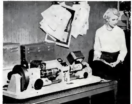
The Fairchild Scan-a-graver Cadet is a table-top machine which uses electronics, optics, and precision mechanics to make plastic half-tones automatically. Designed for the weekly newspaper and job shop, the Cadet makes a maximum eight inch by six inch 85-screen cut in 24 minutes.
