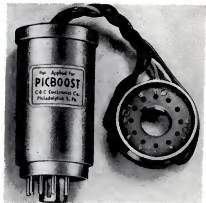
respectively. Models 3F and 4F relieve heater to cathode shorts only, in parallel and series circuits respectively. List price for all models is \$3.25 and dealer net is \$1.95. C-B-C Electronics Co., Inc. P. O. Box 1556, Philadelphia 5, Penna.—TELEVISION RETAILING.
