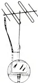
A 6-ft. length of 450 ohm insulated matched strips specifically designed for the use of rotators. Made of Poly-vinyl Chloride. Easy to install at low cost. Eliminates all possibility of shorting out signal. Now, for the first time, your customers can now use rotators for 450 Ohm Open Wire, with all of its inherent advantages.
