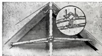
Heavy gauge steel, embossed for extra strength, rust-proof, hot-dip galvanized finish. Upper bracket provides 4" clearance from eave; lower bracket, generous 48" spread. Complete with hardware.
