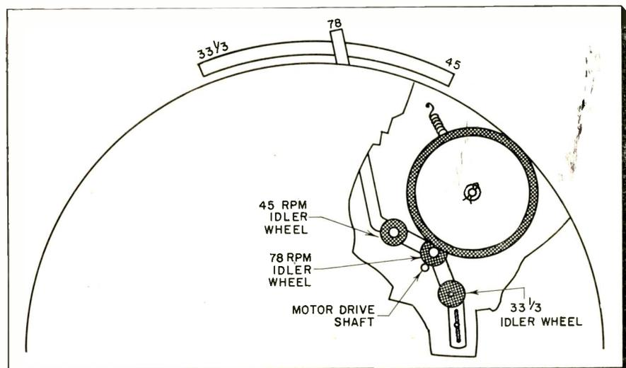
become enlarged due to wear, causing the turntable to rest too loosely on its support; the turntable will tend to slant and scrape the mounting board in consequence. If the spindle wears excessively, a similar condition will be produced.
