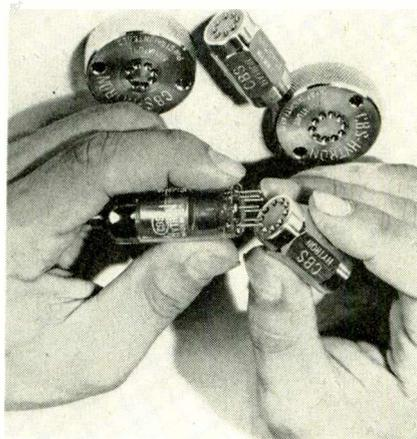
9-pin straightener, mounted back to back. The compact device may be carried in the tool box or in a pocket. CBS-Hytron, Danvers, Mass.—TECHNICIAN
