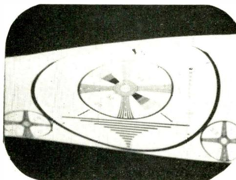
Fig. 7—Vertical keystone effect. Possible trouble sources: Change in value of a shunt resistor across one of the vertical yoke coils; shorted turns in vertical yoke. (Photos on this page courtesy GE; captions based on GE text.)
