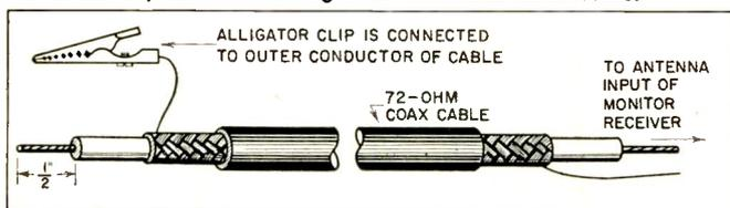
Fig. 3—TVI probe with a wire added to increase its pickup.
