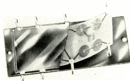
Triple-tie cross-over filter, model UV-3, employs a printed circuit to eliminate the need for two down leads when both a UHF and VHF antenna are in operation. Use of one down-lead eliminates interaction between the UHF and VHF systems, in addition to simplifying the installation job. Impregnation before encasement to make the unit moisture-proof and fungus-proof also eliminates possibility of drift or shorting of components. TV Products Co., Springfield Gardens, N.Y.—TECHNICIAN
