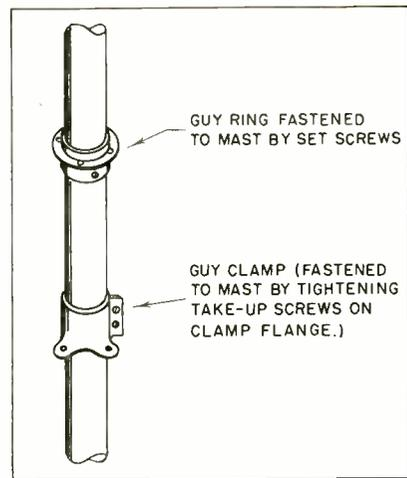
Fig. 3—Methods of fastening guy wires to mast, using either a guy ring or guy clamp.
