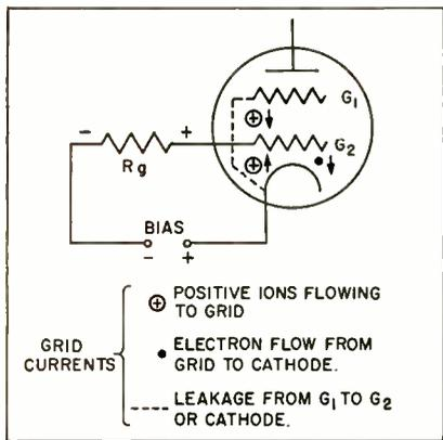
Fig. 1—Gas, leakage between elements ( $G_1$  and  $G_2$ ) and grid emission, may be responsible for lowering the tube bias to the point where cathode emission is destroyed.
