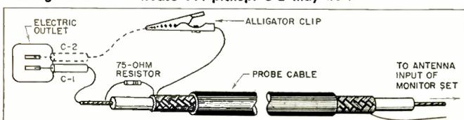
Fig. 5—How an exploring coil is connected to the probe.
