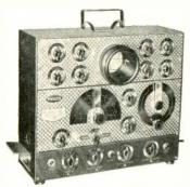
Model 7008—Visual alignment Generator • Combines in one economical unit functions ordinarily found only in a cumbersome collection of costly devices ... Includes extra sensitive built-in oscilloscope ... AM, FM, and audio generators. Sweep output flat to within .2 DB/MC.
