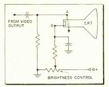
Fig. 2—A cathode-to-grid short in this CRT circuit would reduce the picture tube bias, and also attenuate or eliminate the video signal.
