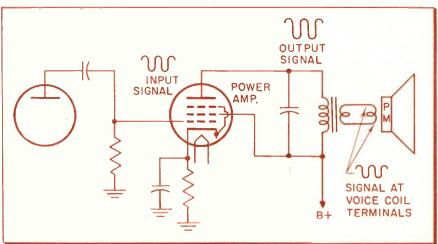
point somewhat clearer. A completely inoperative receiver is checked in a conventional manner by measuring DC electrode potentials at the tube sockets. These potentials appear to be normal. The trouble is actually an open speaker voice coil. A dynamic check would have immediately indicated a discontinuous signal path between the plate of the final audio amplifier and the speaker voice coil (see Fig. 1).
