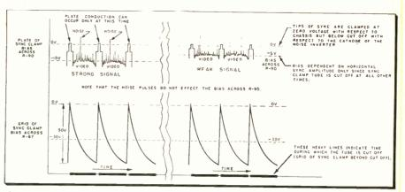
Fig. 3—Waveforms at plate and grid of sync clamper, illustrating why noise pulses **do not** affect the bias supplied to the noise inverter by the sync clamper.
