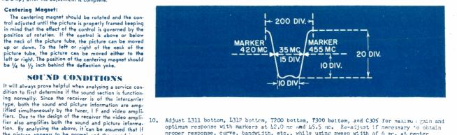
Adjust L311 bottom, L312 bottom, T200 bottom, T300 bottom, and C305 for maximu : gain and optimum response with markers at 42.0 mc and 45.5 mc. Re-adjust if necessary to obtain proper response, curve, bandwidth, etc., while using sweep width of 6 mc. at center frequency of 43.75.
