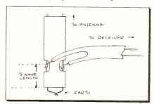
Fig. 4—Using quarter-wavelength of transmission line as a lightning arrester. (Figs. 2, 3, 4 courtesy of Capehart.)
