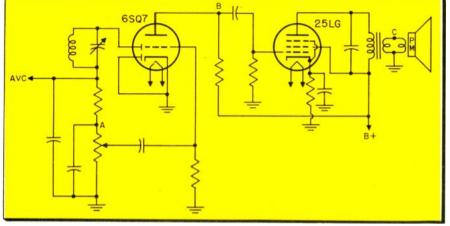
Fig. 2—Initial monitoring setup for intermittent AC-DC broadcast radio receiver. Suggested monitor points are: A and ground; B and ground; C and ground.
