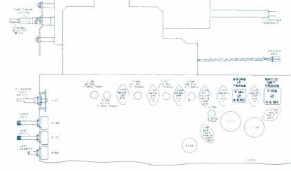
Figure 27-Bottom Chassis Adjustments (KRK29 Tuner Shown)
