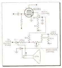
Fig. 3—An increase in the 22K resistor connecting to the brightness cantrol caused an excessive CRT bias, dimming picture and raster greatly. This bias could not be reduced below -30V by manipulation of the brightness control.
