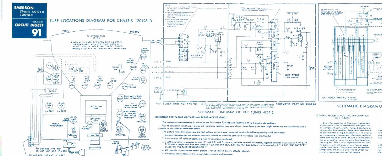
NOTE THE R F AMP TUBE PRESENTLY USED IS A SEKS IN THE FUTURE A SECT. SECTA OR A SET MAY BE USED. THESE THREE TUBES ARE INTERCHANGEABLE, BUT DUE TO POSSIBLE VARIATIONS IN INTERCELECTROSE CAPACITIES, SEVERAL TUBES MAY HAVE TO BE TRIED FOR SET RESULTS.
