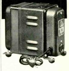
Bad voltage from overloaded lines shifts TV tube operating points and often causes distortion, fuzzy pictures and jitters; high voltages damage components. The SOLA "TeleVolt" Constant Voltage Transformer automatically stabilizes voltage within  $\pm 3\%$ . It automatically protects costly components against high voltage surges while it enables any TV set to deliver peak performance. It is an automatic voltage stabilizer .... not a voltage booster.
