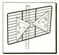
reflector screen and single U-bolt mounting. Snyder Mfg. Co., Philadelphia 40, Pa.—TECHNICIAN.
