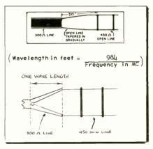
Fig. 3—Methods of matching 450-ohm openwire line to 300-ohm twin lead. Top sketch: the open wire is tapered down to the twin lead over a distance of 30 inches from the first "spreader," as shown. Bottom sketch: 300-ohm line is split over one wave length, and fanned out to the connecting points on the open-wire line.
