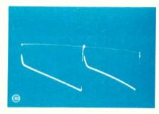
Fig. 2—Actual plate voltage waveforms for the vertical output tube, under the conditions of Fig. 1.
