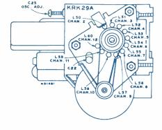
Figure 10-KRK29A/27 Oscillator Adjustments
