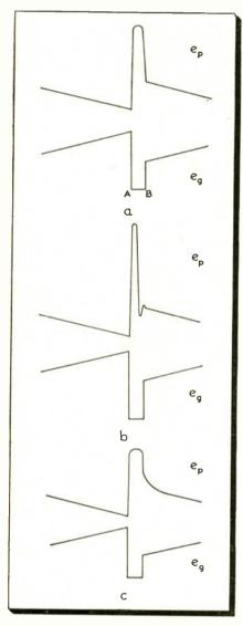
Fig. 1—Vertical output tube voltages. A— Correct peaking; B—Too much; C—Too little.
