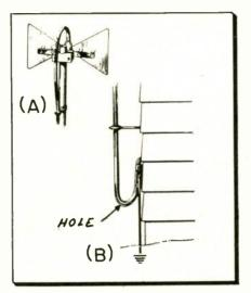
Fig. 2—A) Downward loop is made at antenna when tubular line is employed. B) "Drip loop" is also provided at a point near the one where the tubular line enters the house. A small hole is cut at the point indicated, for drainage.
