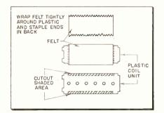
tacts, and remove the coils and forms. Clamp the plastic body of the coil unit in a vise, and file out the shaded areas, within the dotted lines, as shown in the illustration. Cut a piece of hard felt to the width of the filed-out notch. Wrap the felt around the coil unit, fitting it into the filed notches. Pull the ends tight and staple or sew them together. Repeat this job with the second coil unit.
