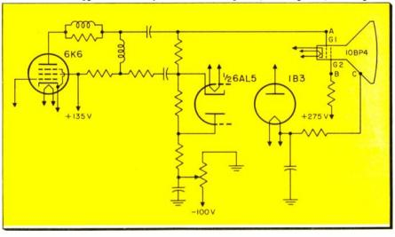
Fig. 3—Initial monitoring setup for TV receiver with intermittent raster. Part of an RCA 630TS circuit is shown. Suggested monitor points are: A and ground; B and ground; C and ground.
