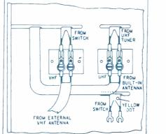
Antenna-Lead Connections, VHF External and UHF Built-In Antennas
