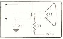
Fig. 5—If R-I in this circuit open-circuited intermittently, a slow fade-out but rapid reappearance of the picture would tend to take place.
