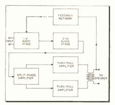
Fig. 4-Block diagram of Hi-Fi Amplifier.
