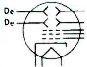
Cathode-ray Tube with Electrostatic Deflection. Remove De for Magnetic Deflection
