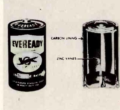
D99 is made to sell for a price slightly higher than standard general-purpose batteries. The zinc electrode of the cell is on the inside, while the carbon is on the outside. This reverses the design of standard flash batteries. As a result, consumption of zinc during use goes on inside the cell. Manufacturer guarantees free replacement of flashlight, if it is damaged by the use of this long-life cell. National Carbon Co., 30 E. 42nd St., New York 17, N.Y.—TECHNICIAN
