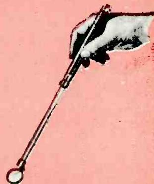
**G-C ILLUMINATED INSPECTION MIRROR** Penlight batteries make this tool independent of cords or connections. Adjustable 1" hinged mirror mounted to 6" transparent lucite rod. No shock. On-off switch. Length 12 1/4". Bulb, less batteries.
