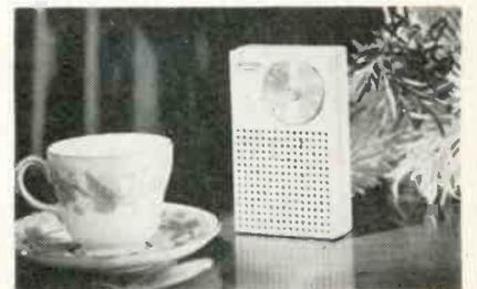
The circuit includes 4 grown junction n-p-n transistors (1 mixer-oscillator, 2 i-f amplifiers, 1 audio amplifier), 1 germanium detector and a tiny 22 1/2-v. battery.
