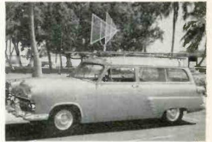
Convinced that TV antennas could best be sold by actual field demonstrations, American Screen Products Co. of Miami outfitted this mobile unit with their Unicorn antenna, a telescoping mast, TV receiver and field strength meter, and sent it out to roam the Florida Gold Coast. The result—discovery of brand new TV fringe areas, and valuable data for local servicemen and TV engineers
