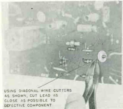
Fig. 1—Avoid soldering directly to the printed wiring by leaving an extra long lead.
