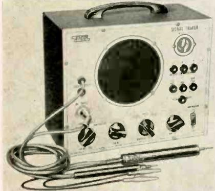
corporates a built-in 5-in. test speaker and magic eye. Exceptionally high r-f sensitivity. Added features include a special Noise Locator Circuit, and a calibrated wattmeter which reveals abnormal wattage consumption in sets under test. Price, in kit form—\$24.95; factory wired,—\$39.95. Electronic Instrument Co., Inc., 84 Withers St., Brooklyn 11, N. Y.—TECHNICIAN (Ask for No. 3-18)
