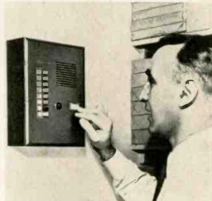
cal central amplifier, rated at 30 watts is the only unit in the system that requires an electrical power outlet. Stations may be installed and full communication provided between as many as six master stations in this new "single conversation" system. In addition to two-way intercom, the system provides complete facilities for paging. Executone, Inc., 415 Lexington Ave., New York 17, N. Y.—TECHNICIAN (Ask for No. 6-27)
