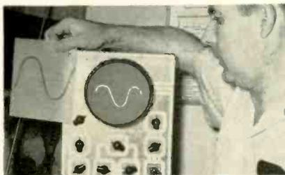
Fig. 2—Input waveform traced on transparent paper, compared to distorted amplifier trace.
