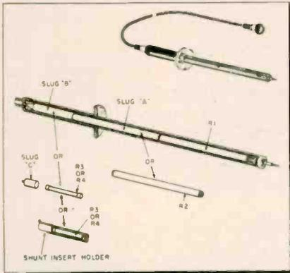
The h-v probe (upper right) and its component parts, showing various arrangements possible.
