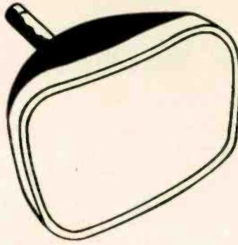
than that used in the face plate. Otherwise, when the neck is heated to seal in the mount, impurities may be given off which could contami-
