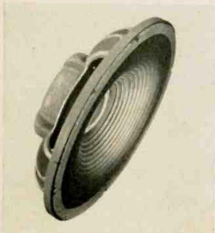
to be mounted between studding, flush with the surface of any standard wall or partition. The unit is not limited to wall mounting; performance improves when enclosed in a reflex cabinet or loaded with a horn. Usable frequency response range, when used as a direct radiator and enclosed with an adequate baffle, extends from 30 to 15,000 cps. Power input is 20 watts and impedance is 16 ohms. James B. Lansing Sound, Inc., 2439 Fletcher Dr., Los Angeles—TECHNICIAN (Ask for No. 7-90)
