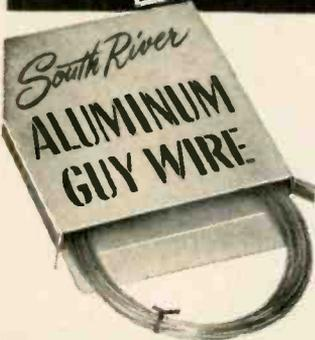
◀ This 7-strand aluminum guy cable of 17 ga. Alclad 56S alloy is specially made for TV guying purposes. It should not be confused with converted clothesline types of cable. Our particular cable has a "tight" twist that gives maximum strength, minimum wind resistance and ice load, does not "basket" when bent. Grey Alclad finish.
