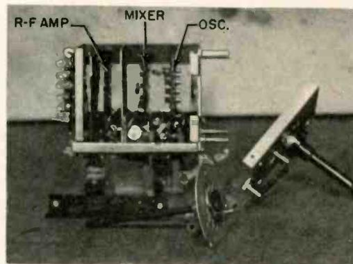
Fig. 5—RCA type KRK-8, shown disassembled, is an "incremental inductance" tuner.
