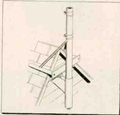
Simply loosen bottom bolt, slip mount into place, and then tighten bolt. Accommodates tubing up to  $1\frac{1}{2}$  in. in diameter. Rohn Mfg. Co., 116 Limestone, Bellevue, Peoria, Ill.—TECHNICIAN (Ask for No. 7-11)
