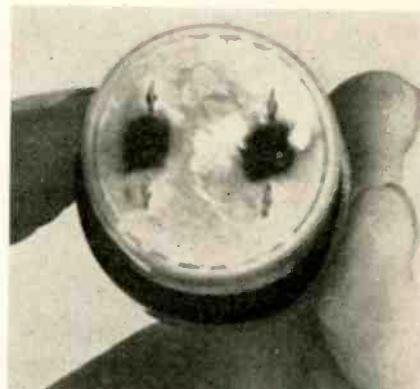
Tube appears new but internal "burn" marks are tip-off that it has seen heavy usage
