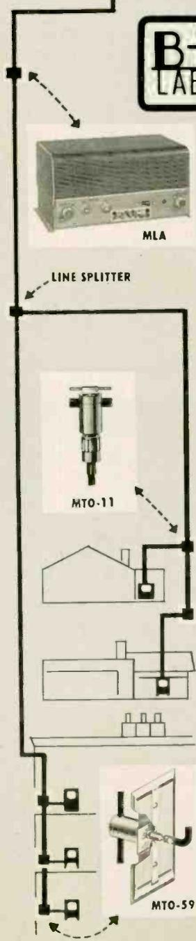
**A** Connect the antenna line to the INPUT of your Masterline MLA Line Amplifier. The signal is now amplified 37db (70 times).
