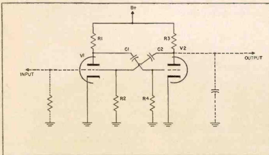
negative, raise or lower tube bias slightly above or below the cut-off point (C. O. in waveform 1). This hastens or retards triggering of the tube, and may thus be said to increase or decrease the frequency of oscillation. This method is generally used when the multivibrator appears as a horizontal oscillator. The dc control voltage is usually the output of the phase detector described in *Let's Look At Circuits, No. 1* (May 1955 TECHNICIAN).
