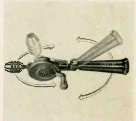
chuck and handle are adjustable to various angles, so that the drill will reach around obstructions, work close to floors and walls, and operate in close quarters: The 0 to  $\frac{1}{2}$  in. capacity chuck swings in a 270° arc, and has a spring lock that enables the user to change angles with a flip of the thumb. The handle turns in a 180° arc at right angles to the chuck movement path. Plomb Tool Company, Los Angeles, Calif.—TECHNICIAN (Ask for No. 7-4)
