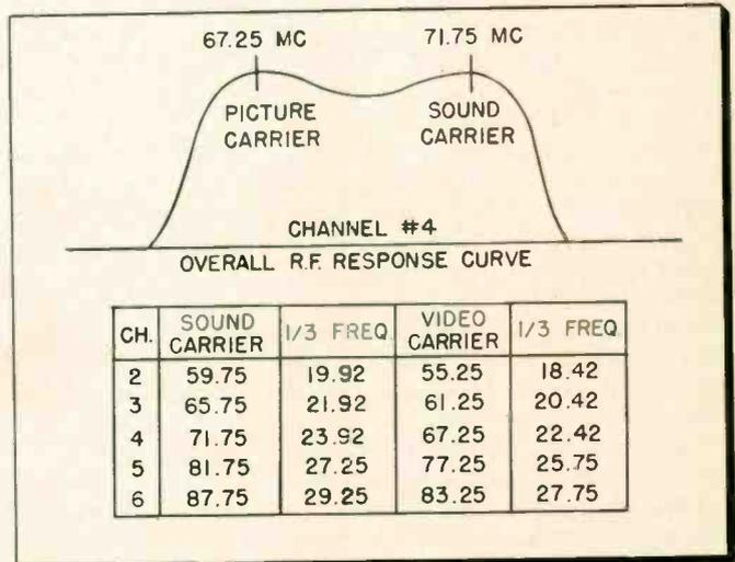
Fig. 6—Carrier pips in Channel-4 response; table for other channels.
