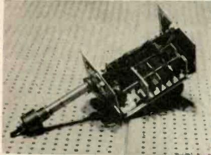
Fig. 7—Variable capacity type tuner has inductances, for low and high bands.
