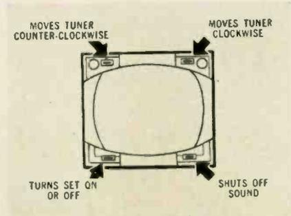
remote control system which permits the customer to change channels, turn the set on and off, or turn down the volume, just by hitting the appropriate photo-electric cell with the beam from the flash-gun provided.
