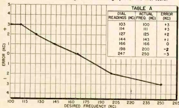
Fig. 4—Table of readings and completed graph for second scale.
