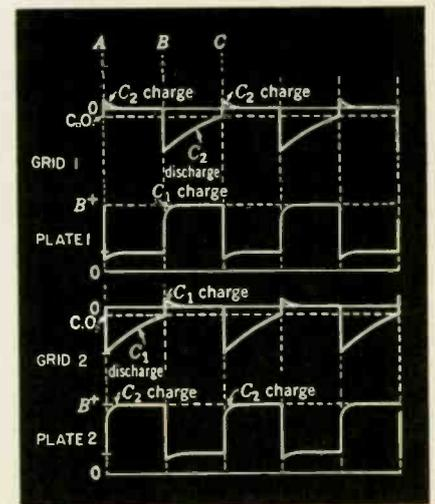
Fig. 2—Grid and plate waveforms for both triodes of a normally operating multivibrator.
