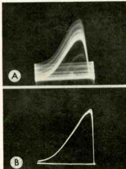
Fig. 5A—Trace blurring caused by stray pickup. B—Lead shielding cleans up the same pattern.
