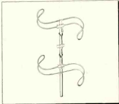
directivity and high gain; is completely assembled. Element assembly to the crossarm is in the Auto-Lock design. The single-bay antenna is Taco No. 644, and the two-bay array is 645. Technical Appliance Corp., Sherburne, N. Y.—TECHNICIAN (Ask for No. 10-39)
