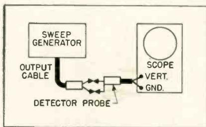
Fig. 2—Arrangement for linearity checking.
