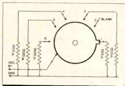
Circuit diagram of handy oscillator tester.
