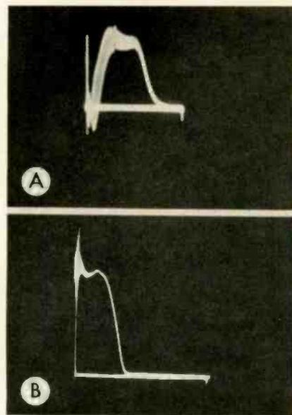
Fig. 3A—Q channel response (to 0.5 mc). B—Response of red amplifier (60 cps to 3.5 mc).
