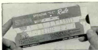
Use this handy pocket-size Sprague Temperature Coefficient Rule to find quickly the values of stock N750 and NPO type ceramic capacitors to connect in parallel to equal a capacitor of desired intermediate temperature coefficient of the required capacitance.
