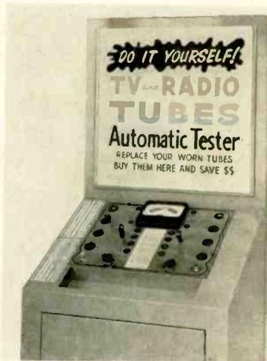
Close-up of Reliable Electronics' newest "Quik-Chek" model shows simplified 20-socket tester mounted on cabinet holding tube supply
