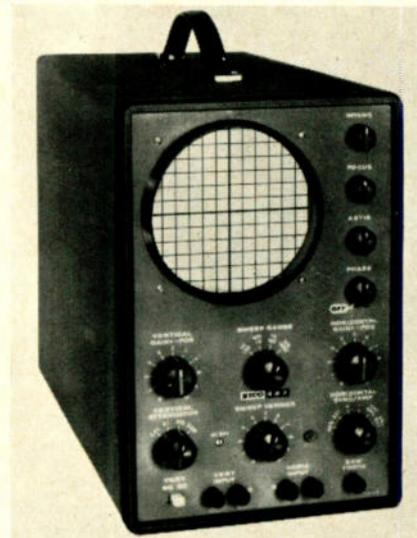
rent sweeps from 10 cps to 100 kc in four over-lapping ranges. List Price \$69.95 in kit, \$109.95 wired. Electronic Instruments Co. Inc.
