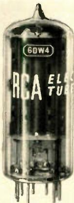
A half-wave no-vari vacuum rectifier tube, 6DW4, is designed especially for damper service in horizontal-deflection circuits of color and BW TV sets. It is rated to withstand a maximum peak plate current of 1300 ma and a maximum d-c plate current of 210 ma. Has insulation between heater and cathode to withstand negative peak pulses between the heater and cathode of 4500 v with a d-c component up to 900 v RCA, Electron Tube Division.
