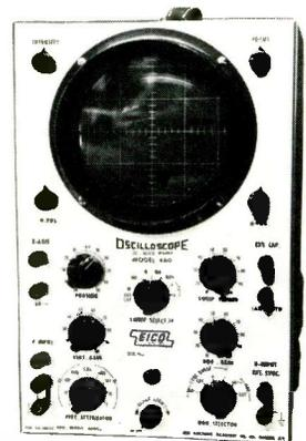
Eico Model 460 dc oscilloscope.
