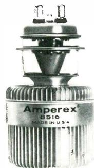
tetrode of the 3 kw plate dissipation class designed for use as an RF amplifier for frequencies extending throughout the VHF range. Both the control grid and screen grid connections are made to ring-type connectors brought out through the tube envelope. This facilitates operational performance by eliminating discontinuity in the impedance versus frequency characteristics. Amperex.
