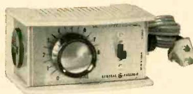
G-E electronic speed control lets low cost power tools do work of costly more powerful tools. Use at work or home for any universal motor-driven tool with nameplate rating up to 5A, 120V, ac. Particularly good for resistive type soldering irons to give low-heat tip temperatures for printed circuits. Order ETR-3921.
