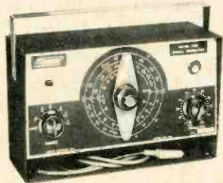
TV and communications equipment is announced. The model 1500 has a separate high level audio output for checking Hi Fi sets and video amplifiers. The unit provides seven overlapping bands, 115 kc to 110 Mc to cover frequencies required in normal service work. A panel slide switch changes the generator output from a RF sine wave to 400 cps AM modulated RF, each with control for adjustable output level. Mercury.
