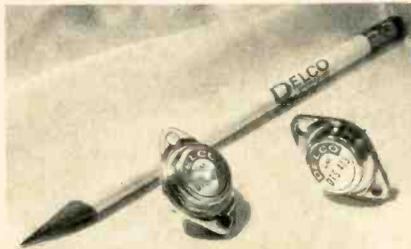
factory operation of the horizontal output stage with a semiconductor device has been a major problem in the design of solid state, large screen TV, both technically and economically. Development of an advanced silicon wafer technique known as the triple sequential diffusion process will permit low cost volume production of the devices. Delco.
