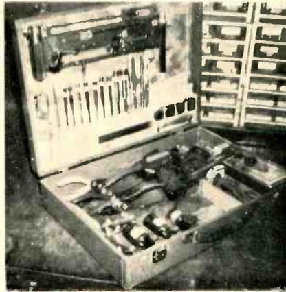
Attache case may be converted into a functional tool box.
