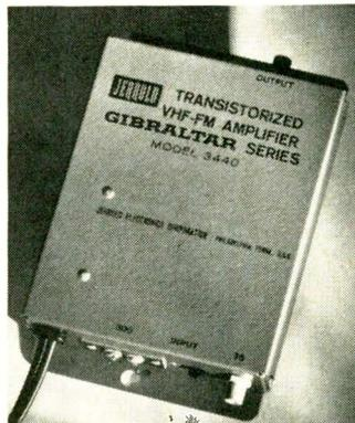
Heart of the system is the new solid-state GIBRALTAR amplifier. Low noise figure (less than 6 db) means GIBRALTAR works well even in weak-signal areas. High output capability (more than 150,000 microvolts) lets it work in very-strong-signal areas without overload. High gain (25 db avg. hi band; 23 db avg. lo band and FM), consistent performance and maintenance-free reliability make GIBRALTAR the ideal amplifier for every small VHF system you install.
