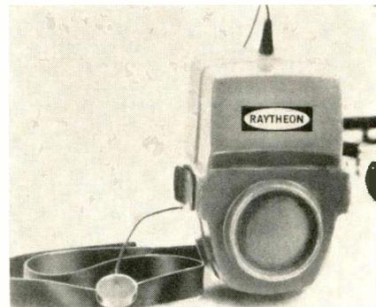
and a sound diffuser to eliminate bubble sounds and a plastic case containing the amplifier circuitry, dry cell battery, and speaker. The microphone assembly fits inside an ordinary diving mask while the speaker case is worn on the weight belt. The complete system weighs 25 oz in the water. Raytheon.
