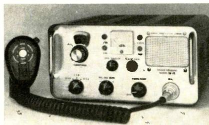
cluding compactrons and nuvistors. It has a built-in power supply for 12 or 115v operation. The unit is an upper sideband, lower sideband or double sideband transceiver. General.
