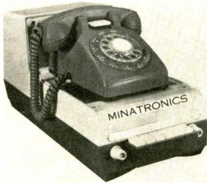
taining high quality throughout. High fidelity tape recorders transmit voice recordings and record messages left by caller, according to the manufacturer. Minatronics.
