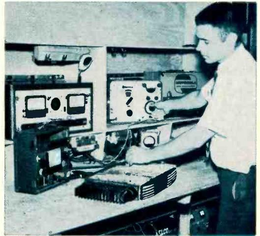
Technician Goodell aligns receiver of transistorized mobile unit in field maintenance shop.
