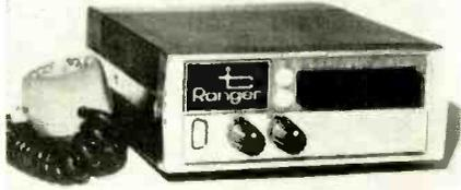
output of 3.7w with 85% upward minimum modulation, the manufacturer says. A base station console is available for use with transceiver. Texas Communications.
