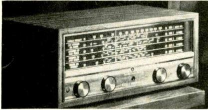
nounced. The receiver provides coverage of the 5.9-6.25 MC (49 meters); 9.45-9.8Mc (31 meters); 11.65-12.05 Mc (25 meters); and 15.05-15.55 Mc bands. These bands are in addition to the standard broadcast band of 550-1600kc. Sizes 13½ by 5¾ by 8¾ in. Hallicrafters.
