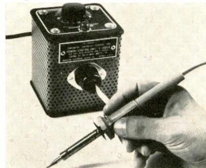
ing iron which utilizes regular tips is announced. The power-control unit's range of 350-750° tip temperatures is set by a direct-reading dial. American Beauty.
