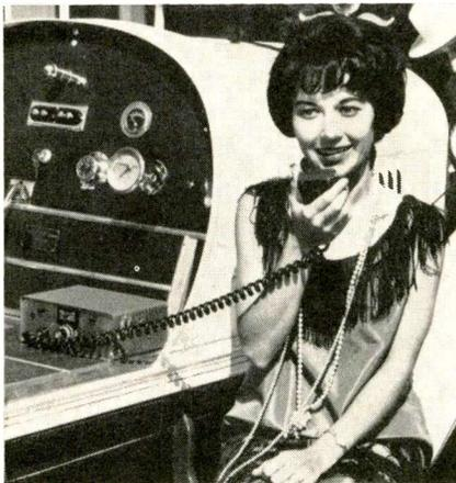
than one cubic ft. In addition to operating as a two-way CB radio, the unit may be used as a public address (PA) system with 3w audio-power output and includes a jack for external speaker connections. The unit requires a 12vdc power supply with either positive or negative ground. RCA.
