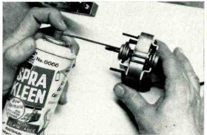
Cleaning motor bearings with bearing-plate removed.
