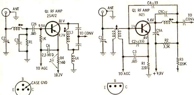
Fig. 1—(Left) Model 235, 1965 Dodge germanium RF stage. (Right) 1966 Dodge silicon RF stage from model 2355 radio.
