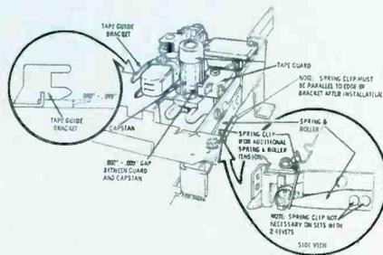
Fig. 6—Details for adding spring clip if additional tension is required to detent cartridge properly.
