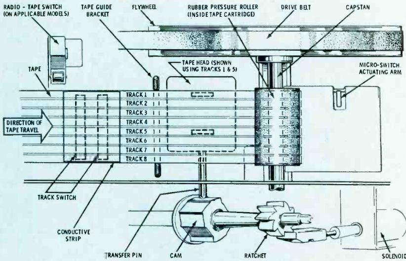
Fig. 4—Tape drive and head positioning details of Motorola tape-player.
