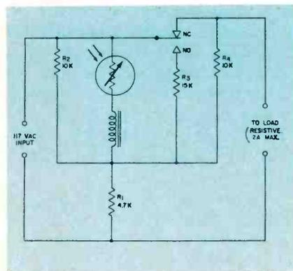
Fig. 3—Dusk-to-dawn automatic lighting circuit using photoconductive cell. Courtesy of Sylvania Electric.
