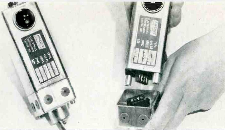
Interchangeable plug-in photoelectric controls by Frost Electronics.
