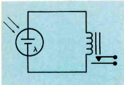
Fig. 1—Basic photovoltaic relay circuit.
