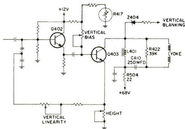
tance. During retrace time, a large positive pulse is developed by L401 which reverses the current through the yoke and moves the beam from the bottom of the screen to the top.
