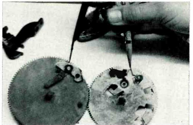
Pawls must be kept free of lubricant. Kept free of all foreign matter these mechanisms will operate for long periods with little attention.
