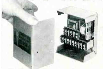
Transistorized photoelectric relay by Farmer Electric.
