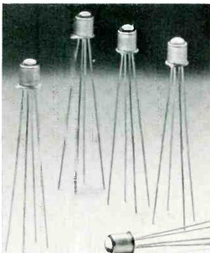
Light sensitive field-effect transistors by Crystalonics Inc.
