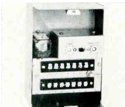
Modularized photoelectric control system by Photomation.
