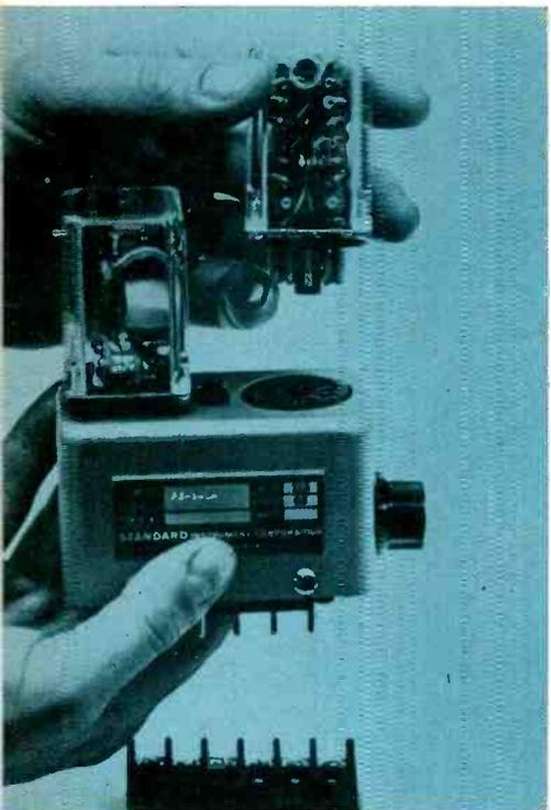
Transistorized 'plug-in' photo-electric control by Standard Instrument.
