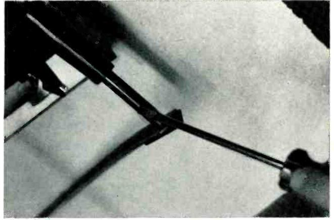
Fig. 3—The leveling arm is always moved by grasping it at the rear—not near the spindle end.
