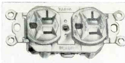
unit from hazardous penetrating elements. Phosphor-bronze, steel-reinforced contacts are enclosed in individual recesses. The contacts are a double-grip type designed for 8 lb pull without detent. This device is not recommended for installation in unprotected outdoor areas. Pass and Seymour.
