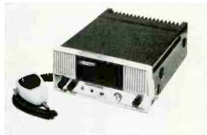
output is 5w with less than 5% distortion. Plug-in channel elements provide one through four channels. The tone-coded squelch option reduces the possibility of hearing other systems that share a channel. The radio is also designed for easy field conversion to split-channel operation when such changes are required. Motorola.
