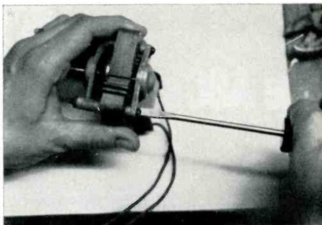
Fig. 1—The screws holding the bearing plates can be adjusted for correct alignment.
