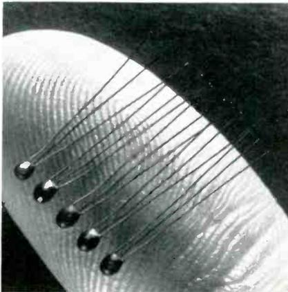
strumentation, hybrid circuits, linear and analog circuits, miniature operational amplifiers, or any other application where small size is important. The amplifiers are color coded for type number and lead configuration. Package size is 0.07 x 0.07 x 0.085in. G-E.
