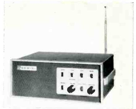
is announced. As an FM alerting receiver, the unit remains on silent standby until activated by a tone signal transmitted from headquarters. It can then receive voice messages at full sensitivity. The receiver is offered in the low (30 — 50MHz) or high (150 — 174MHz) bands with other frequencies available on special order. A number of optional features are available. Viking Inst.
