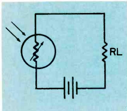
Fig. 2—Simplified photoconductive cell relay circuit.
