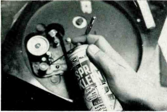
Fig. 2—Motor bearings can frequently be cleaned without removing the motor from its mounting position.
