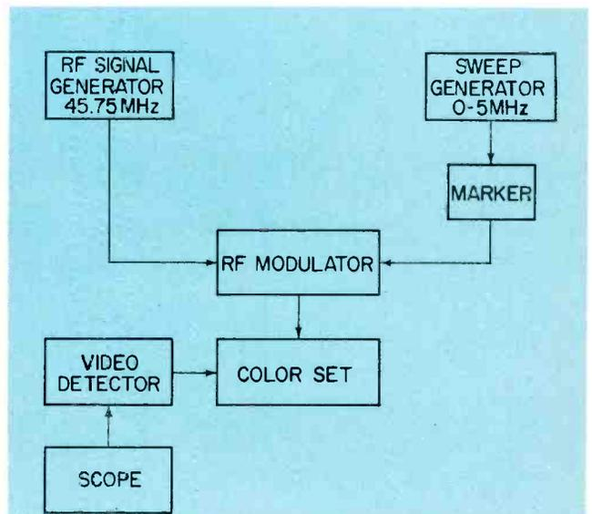
Fig. 5—Block diagram of chroma alignment setup.
