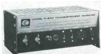
hard-to-start loads, an indicator light which shows the battery's condition and warns when the output is shorted or overloaded, plus automatic electronic overload protection. Voltage regulation is 11% of no-load voltage, and frequency regulation is 4Hz from no load to full load. Dimensions, 4½ x10x7½ in. Weight, 9 lb. List price, \$89.50. Electro Products.
