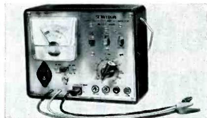
age. It can be used as a circuit signal generator or tracer, measure supply voltages on a 20-v scale and measure current drain to 100ma. Semitronics.
