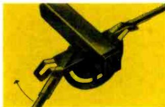
The wedge-snap lock actually tightens and improves with vibration. The spring pressure of the clamp jams the wedge aperture over the squared dipole's end. Since it cannot seat all the way down, a sharp pressure is maintained on the edges of the dipole. Vibration merely tightens the pressure, jamming the wedge into the dipole so that it is both self-cleaning and self-tightening.
