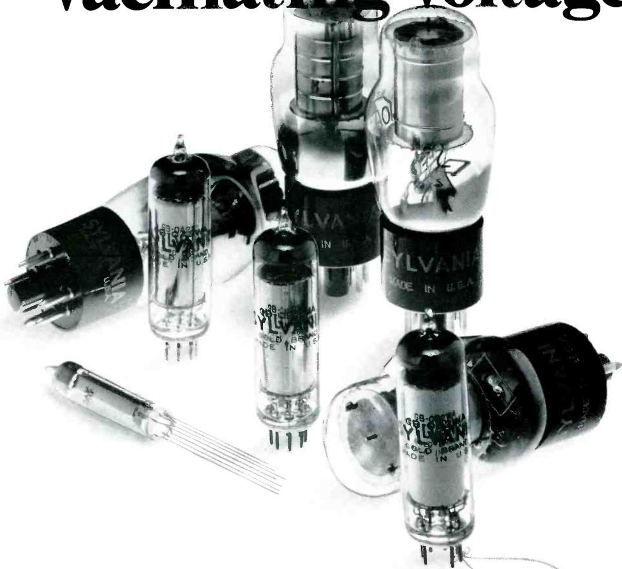
For better regulation and other electrical characteristics, choose from Sylvania's broad line of cold cathode, gas-filled Voltage Regulator tubes. You'll get the benefit of continuing improvement in tube design and manufacturing techniques.
