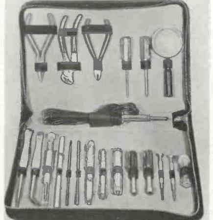
tronic equipment. The manufacturer indicates that these tools include one chain-nose plier, groove-grip plier,
