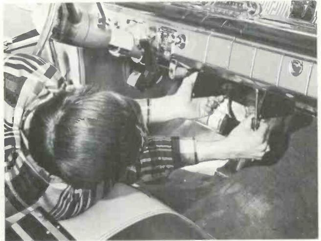
Fig. 3 — Mount the bracket tight against the metal underdash in a clear area.
