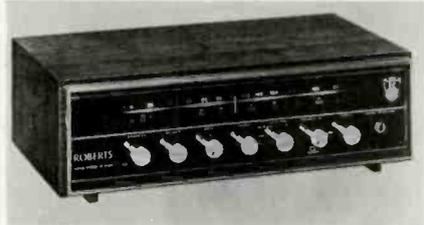
record changer. Specifications indicate that the receiver has a controlled injection AFC, a broad-scale logging dial all solid-state circuitry. Rheem.
