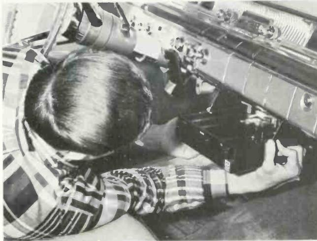
Fig. 4 — The tape player is easily removed by unloosening the two side bolts.
