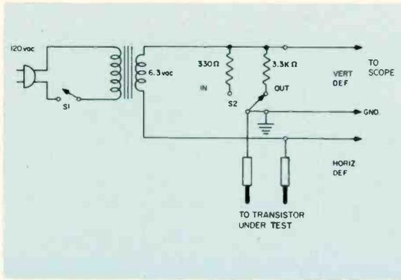
Fig. 8--Schematic of the transistor or diode tester.
