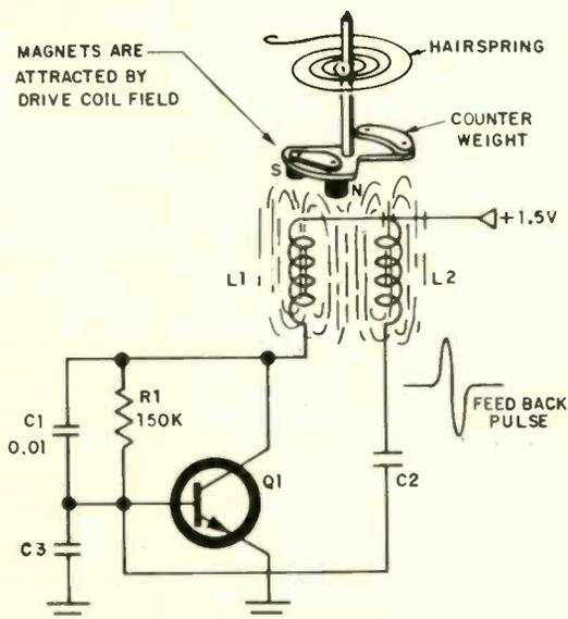
circuit to drive the clock mechanism. The transistor clock circuit closely resembles a blocking oscillator. In place of
