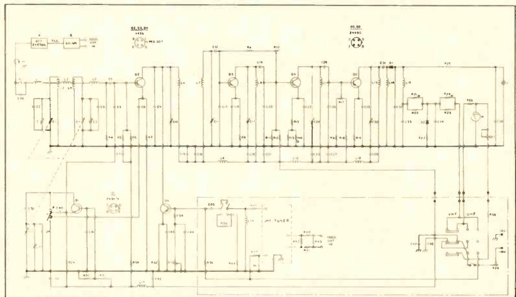
Fig. 3--Schematic diagram of SSM model 718 (Courtesy Jerrold).
