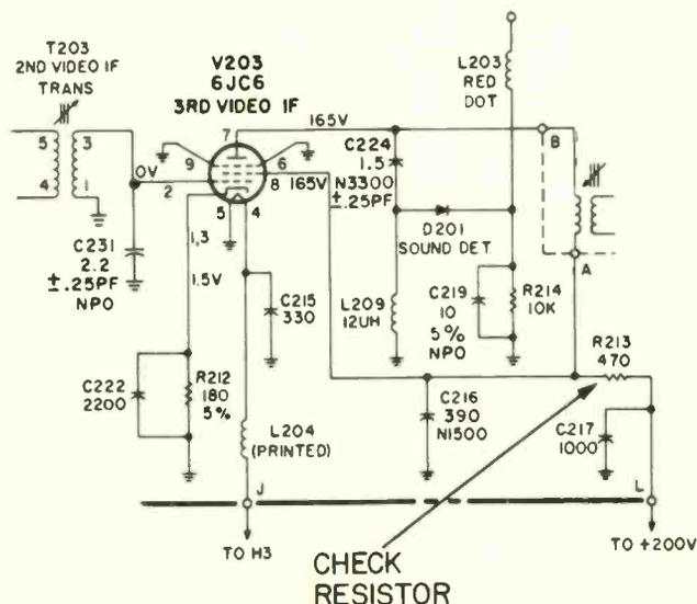
ptoms are noted. Sometimes the failure of the 6JC6A 3rd video IF tube will result in failure of the plate/screen load
