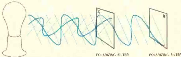
Fig. 5--Polarizing filters can be employed to stop virtually all light when they are rotated out of phase.
