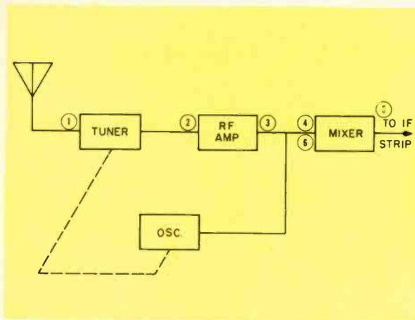
Fig. 8--Block diagram of typical TV RF section.
