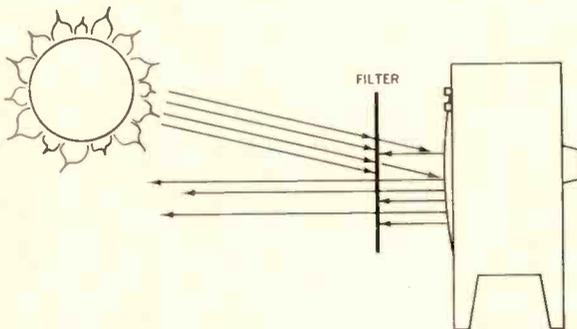
Fig. 3--A 50 percent transmission filter demonstrates how only 25 percent of the reflected light is seen but 50 percent of the phosphor light is seen.
