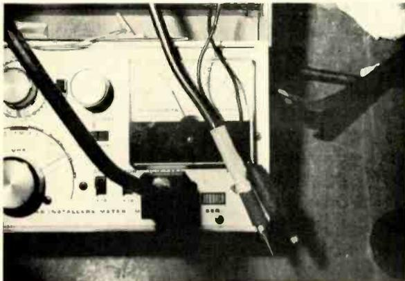
Fig. 6--Shows completed probe used for signal tracing.
