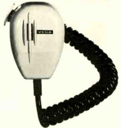
intelligibility. The standard model operates from 10.5 to 18vdc between -30 and +65°C, and has attack time of 1ms, released time of 0.25s and harmonic distortion of less than 5% over full compression range. Vega Electronics.
