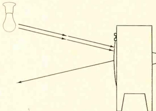
Fig. 1--Reflected light allows you to see the screen when there is no light from the set itself.
