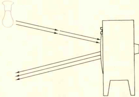
Fig. 2--When the set is turned on, light from the phosphor overpowers the reflected light and makes the screen appear black.
