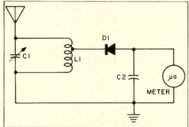
Fig. 2--Simplified schematic diagram of SSM circuit.
