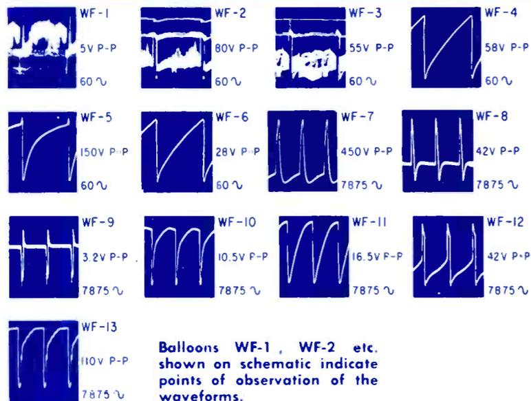
Balloons WF-1, WF-2 etc. shown on schematic indicate points of observation of the waveforms.
