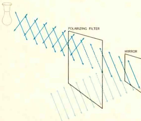
Fig. 6--When light is reflected from a smooth surface, the angle of polarization is not reversed.
