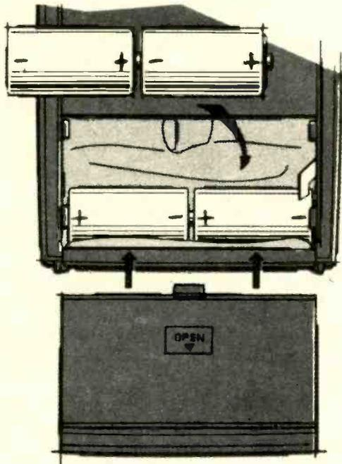
battery outline provided on the plastic pull-out tab. This will result in jamming of the tape in the PLAY or RECORD positions.
