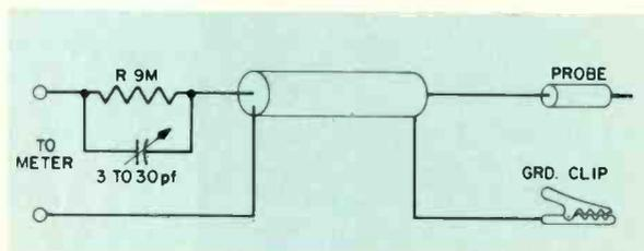
Fig. 7--Schematic diagram of low capacity probe which can be used to reduce circuit loading.
