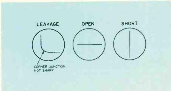
Fig. 4--Three basic waveforms produced by a defective transistor.
