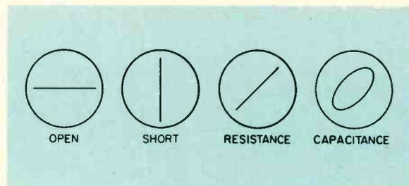
Fig. 1--Basic waveforms that are obtained from pure circuit load checks.
