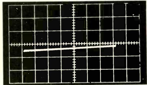
Fig. 7--A normal waveform taken from the emitter to collector of transistor.
