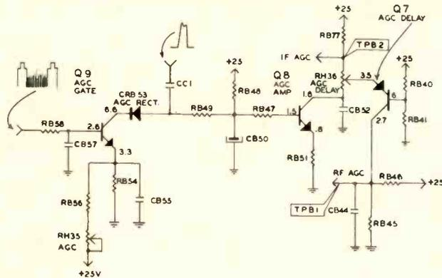
an RC isolating network. The base emitter junction is reverse biased but the sync pulses are of sufficient positive amplitude to drive the base positive and cause the transistor to conduct.
