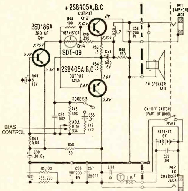
circuit board just to the left of the speaker magnet. If the control is defective, moving it usually causes the distortion to be intermittent. The problem is a poor connection where the lug is riveted to the control element—we suggest replacement of the control. The replacement control must be adjusted according to the procedure given in service
