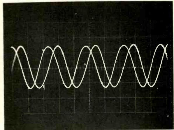
Fig. 8--A dual-trace triggered scope waveform of the CW signal. The 3.58MHz CW signal had been superimposed on the scope for an exact phase check of the 104deg signal shift.
