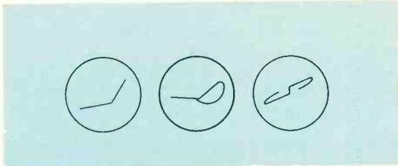
Fig. 3--In-circuit checks will display waveforms shown for a good semi-conductor or diode.
