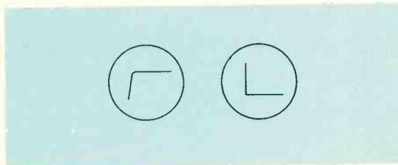
the transistor. Most base to emitter or collector tests of a good transistor will indicate a typical diode pattern as shown in Fig. 5.
