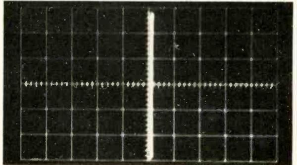
Fig. 11--Waveform showing a shorted transistor.
