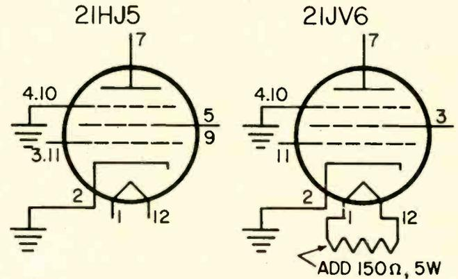
13GB5 tube, which replaced the 21HJ5 in later runs of these chassis, has been suggested as a substitute. However, this substitution required changing the tube socket and other components. We can now supply the 21JV6 which will replace the 21HJ5 with only slight rewiring of the original socket and the addition of a resistor across the heater.
