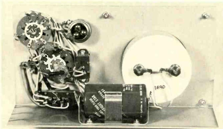
Model IT-18 in-circuit/out-of-circuit transistor tester measures gain (beta) and leakage. The circuit is basically a low impedance, common-emitter amplifier using the transistor being tested to complete the circuit.
