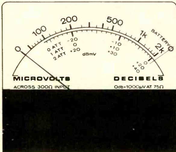
Fig. 1--Typical signal strength meter face reads dbmv and microvolts.
