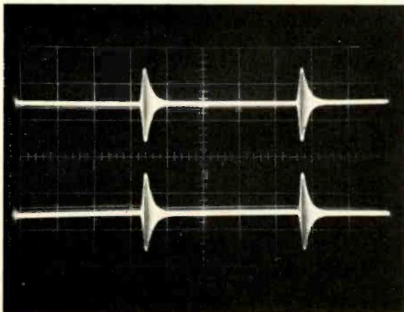
Fig. 5--The dual-trace oscilloscope waveform shows a balanced 3.58MHz color burst signal taken at the secondary of the AFC and ACC phase detector transformer.
