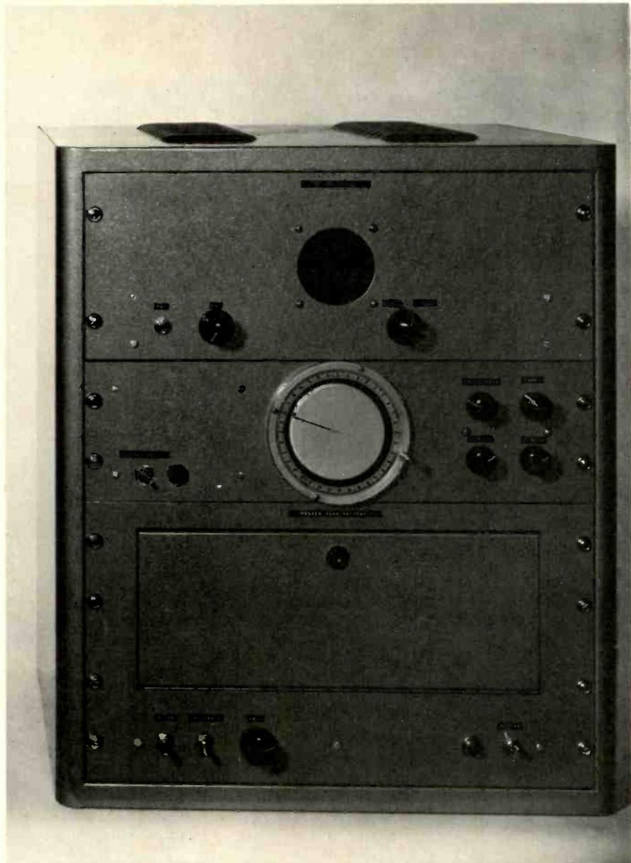
Cathode ray tube lightning detector (Courtesy British Columbia Forest Service)
