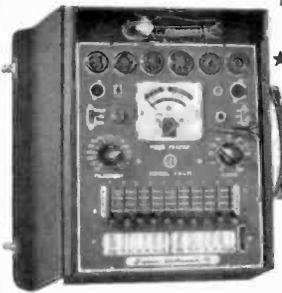
★ Tests all tubes, including 4, 5, 6, 7, Octal, Lock-in, Hearing Aid, Thyatron, Miniatures, Sub-miniatures, Novals, Sub-minars, Proximity fuse types, etc.
