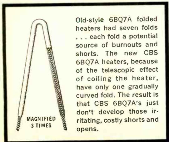
Old-style 6BQ7A folded heaters had seven folds . . . each fold a potential source of burnouts and shorts. The new CBS 6BQ7A heaters, because of the telescopic effect of coiling the heater, have only one gradually curved fold. The result is that CBS 6BQ7A's just don't develop those irritating, costly shorts and opens.
