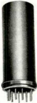
band transceivers. Provides increased d-c output from the rectifier, and better regulation and high reliability. No filament power is required. \$13.00. Sarkes Tarzian, Inc., Semiconductor Div., 415 N. College Ave., Bloomington, Ind.
