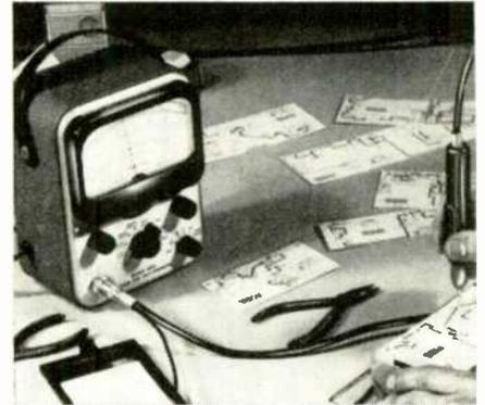
cuit paths and printed locations of major components that match various chassis in the firm's transistor radio line. Visual identification is made of the r-f, i-f, and audio signal paths antenna to speaker. Voltages, and component data are included. Philco Corp., Tioga & "C" Sts., Philadelphia 34, Pa.
