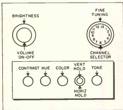
Fig. 1—Customer-operated controls on front section of typical color TV.
