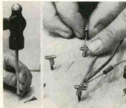
connector and the time-saving "drive in" design which provide an ideal combination for use in making all kinds of harness cable assemblies. Will not bend, pick, balloon or damage leads. Easy to mount on board with hammer and simple driving tool. No drilling or counterboring required. E-Z Hook Products, 1536 Woodburn Ave., Covington, Ky.
