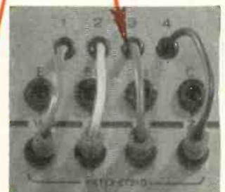
Precision's "Patchcords" setup tests test sockets' pin connections. Dual jacks permit great test flexibility for uncommon transistors.
