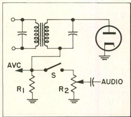
avc voltage and sets the point at which limiting begins. Audio across the volume control R-21 is fed to the first audio amplifier.
