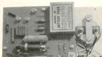
gain readings from transistor manual. Unit has signal injection facility. Rich harmonic signal can be adjusted with attenuator control. Also provides signal tracer with volume control.
