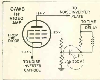
In many RCA Color TV receivers a  $2\mu\text{f}$  filter capacitor, mounted on the video amplifier printed board may cause a variety of annoying picture symptoms.
