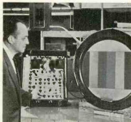
Hickok Electrical Instrument Co's NTSC standard color bar generator produces a pattern of seven colors for accurate adjustment of color TV receivers.
