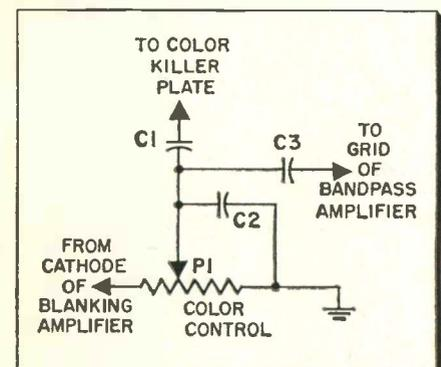
Operation of the color control is shown in Fig. 3. Positive pulses from the blanking amplifier cathode are fed to the band pass amplifier's grid. When the color control P1 is turned toward its grounded end, the positive voltage to the band pass amplifier grid decreases. Thus, the amplifier gain is reduced. Turning the control in the opposite direction, of course, has the opposite effect.
