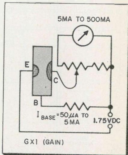
Fig. 2—Basic current gain test-circuit for Precision's model 960 tester.
