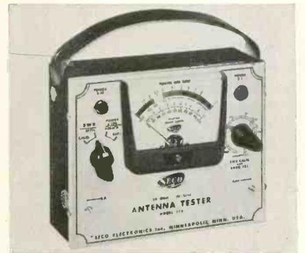
Can also be used as an in-line r-f power meter. Has 3 ranges, 0-10 watts; 0-100 watts; and 0-1000 watts. Dial scale, calibrated from .5 watts to 10 watts full scale. Standing wave ratio scale from 1:1 to 8:1. Accuracy, ±5% at full scale. Indicating meter, 80 μ amperes full scale. \$42.95. Seco Electronics, Inc., 5015 Penn Ave. S., Minneapolis 19, Minn.
