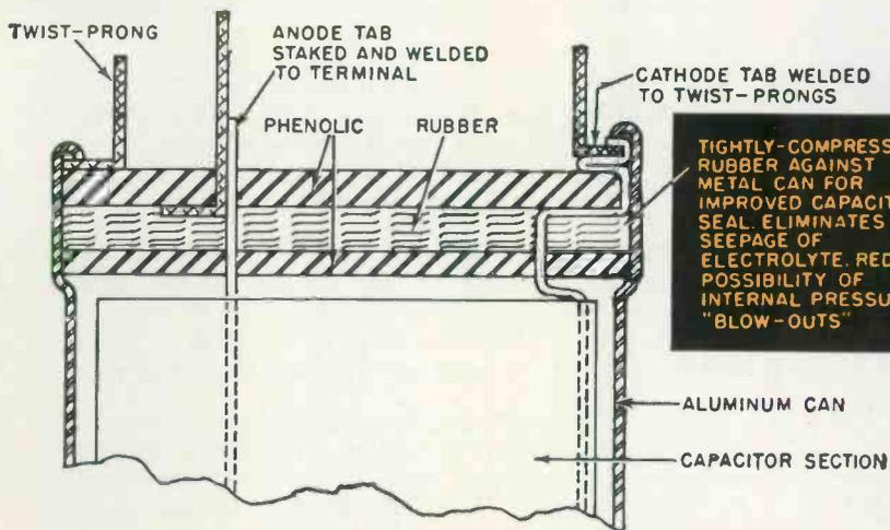
TIGHTLY-COMPRESSED RUBBER AGAINST METAL CAN FOR IMPROVED CAPACITOR SEAL. ELIMINATES SEEPAGE OF ELECTROLYTE. REDUCES POSSIBILITY OF INTERNAL PRESSURE "BLOW-OUTS"
