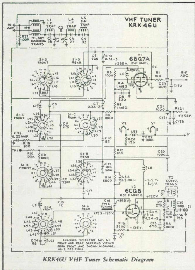
◀Fig. 1—Schematic diagram of an RCA KRK 46U VHF TV tuner. Snowy pictures, pix pulling, and absence of audio or video, may be caused by a tuner's mechanical or electronic defect.
