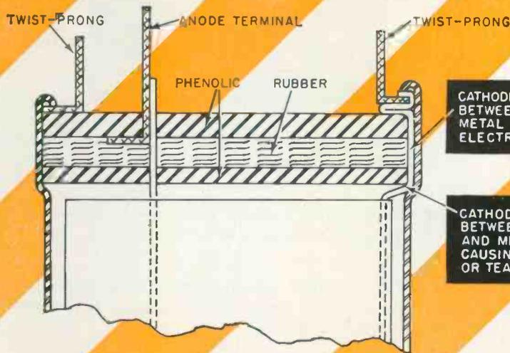
CATHODE TAB BREAKS SEAL BETWEEN RUBBER AND METAL CAN, PERMITS ELECTROLYTE SEEPAGE
