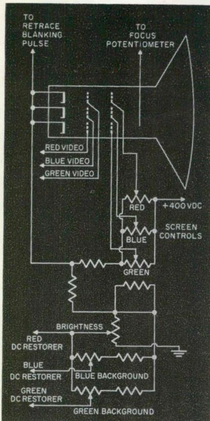
Fig. 4—Screen and background controls in typical CRT circuitry of color TV.
