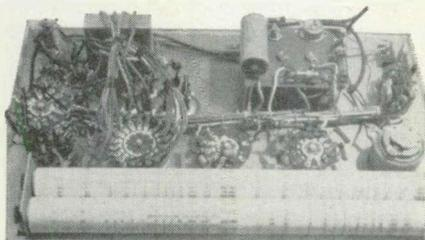
has a 100  $\mu$  ammeter. Variable controls, though not as broad as the \$298 Hickok's range, is wide enough to simulate typical operating conditions. A roll chart lists all essential test set-up information. One-year free test data is provided; a nominal charge for renewing this service, optional, (\$1.25 each). Tester has a line voltage adjustment to assure measuring accuracy.
