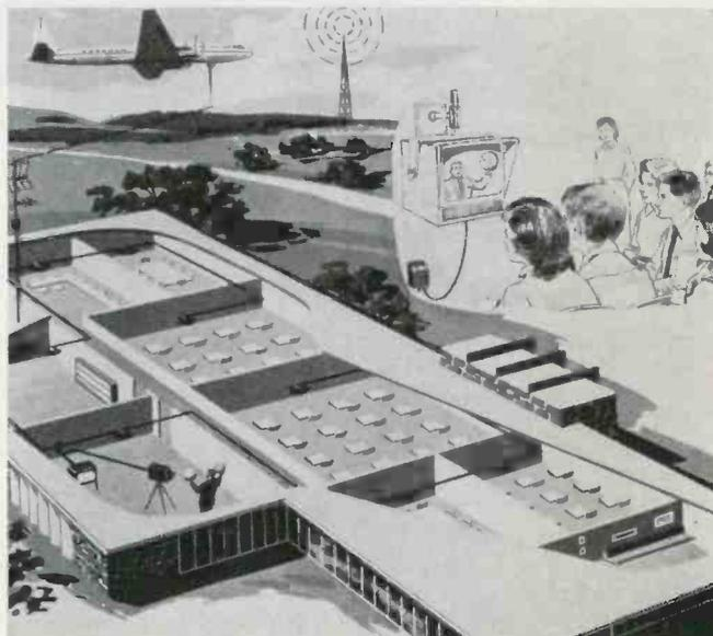
This is a typical Jerrold installation for educational TV in the MPATI area (Midwest Program on Airborne Television Instruction). Circling aircraft transmits two videotaped courses over channels 72 and 76 to school. Signal is converted to VHF, amplified and distributed through school by coax to standard receivers. System provides for closed-circuit TV.
