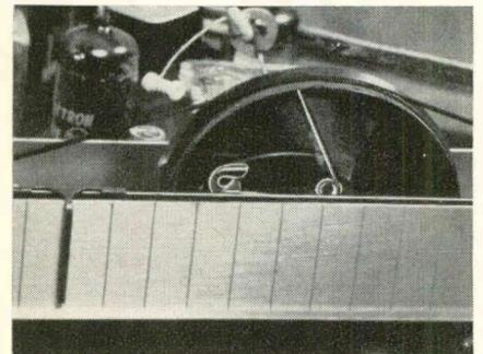
A large safety pin can replace the drive pulley's spring in an emergency. See Text!
