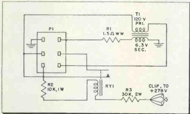
Building this substitute power box will enable technicians to offer a customer use of his remote-tuned GE TV set when the remote receiver chassis needs shop work.
