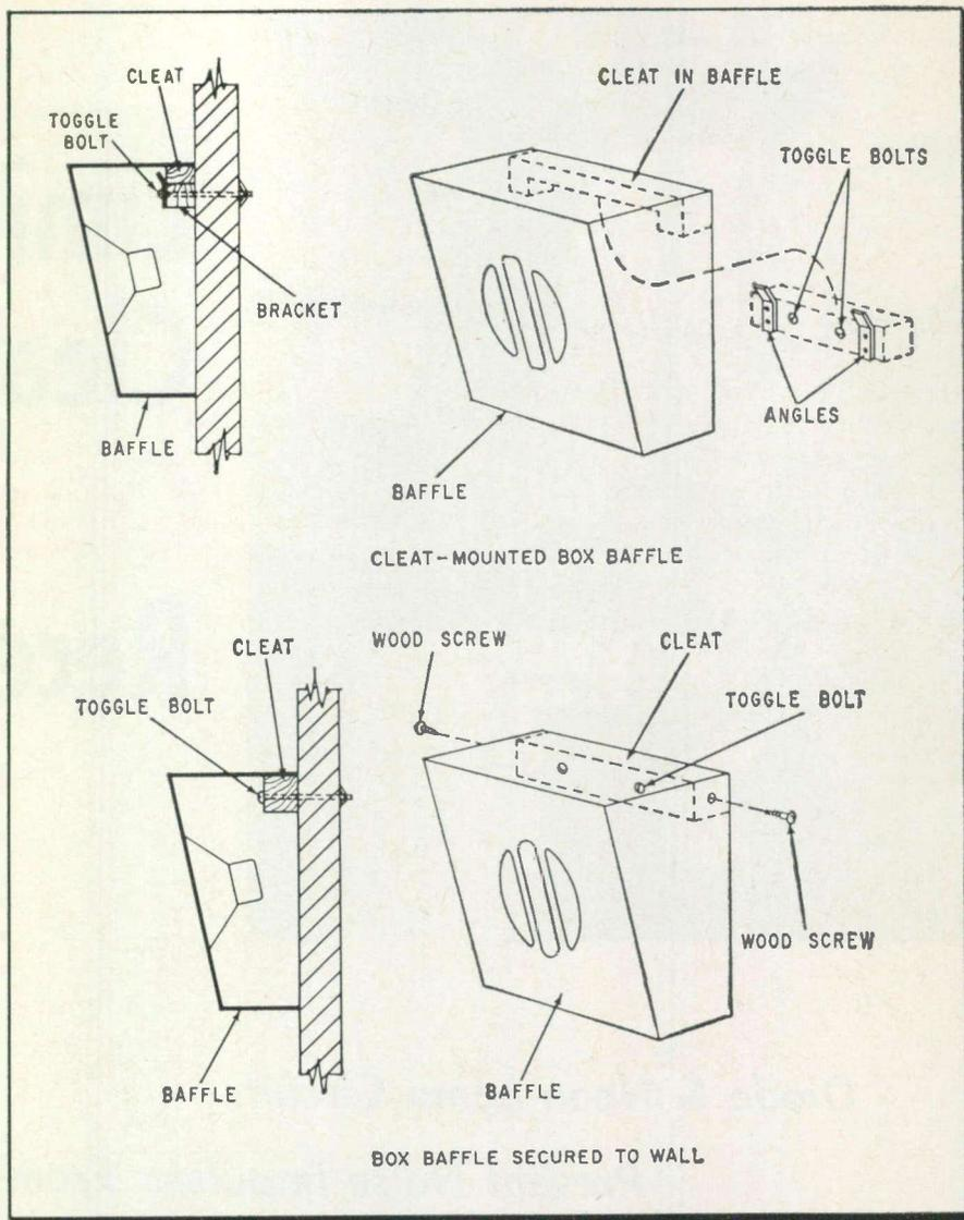
Fig. 4—Speaker box baffles can be easily secured to any type wall with cleats.
