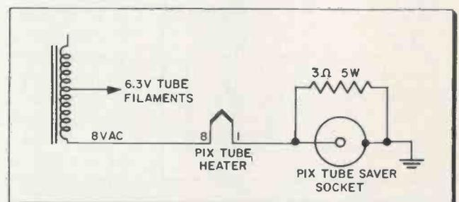
This set has a built-in CRT booster! Filament voltage can be increased from 6.3 to 8.2 volts by shorting out a resistor.
