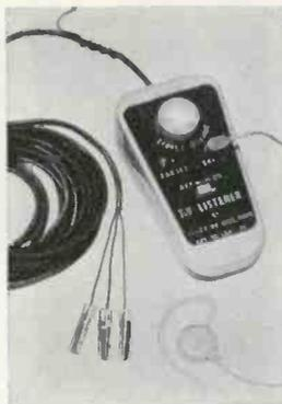
Clips permit simple and safe attachment to TV or radio. Earphone has 5-foot cord and Listener has a 15-foot flexible cord. \$14.85. Telex Inc., Telex Park, St. Paul 1, Minn.
