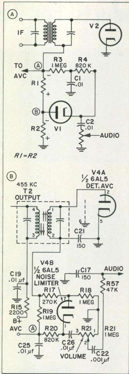
Fig. 2 (A)—Actual series noise limiter circuit with vacuum tube diode acting as a switch to keep noise pulses from the audio. (B) This same circuit as it appears in a popular Citizens Band unit.
