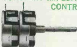
Self-compensating L-pads and T-pads rated at 10 watts audio. Continuous range from 0.5 to 30 db attenuation.
