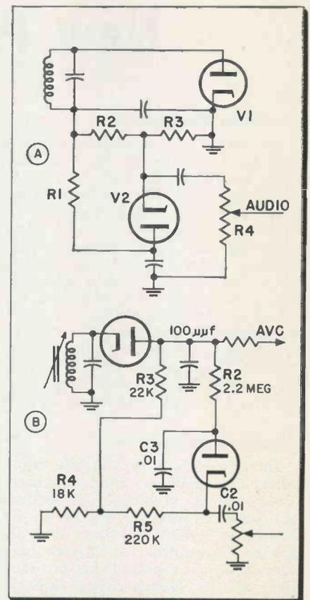
Fig. 3—Examples of shunt type noise limiter circuits. In circuit A, V<sub>2</sub> only conducts on noise pulses when its cathode is more negative than its plate. Limiter B utilizes the long time-constant of R<sub>2</sub> and C<sub>3</sub> to keep noise pulses out of the audio output circuit.
