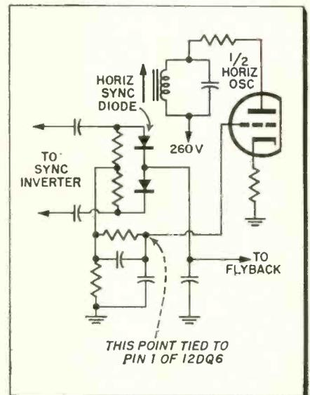
High resistance leakage between the horizontal output tube heater and phase detector caused picture weaving on an Admiral TV.
