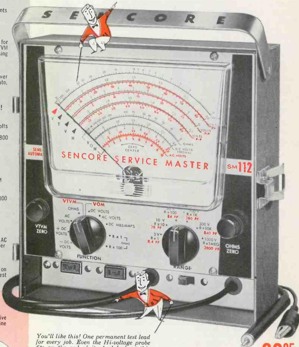
You'll like this! One permanent test lead for every job. Even the Hi-voltage probe fits on the end of it. And look at this storage compartment for test lead and line cord. The two 115 volt AC outlets sure come in handy on service calls!
