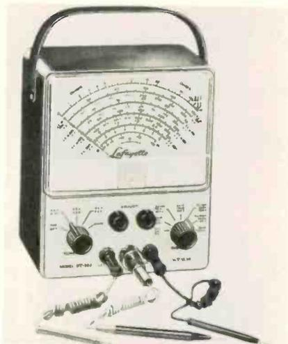
up to 2000 volts on any wave form from 30 cycles to above 5 mc, without using accessory probes. Direct resistance measurements on ohms scale from 0.2 ohms to 1000 megohms and decibel scale range from -10 to +15 with db readings possible to +58 db plus a zero center scale. \$25.95. Accessory r-f probe is optional for KT-202 or any other VTVM, KT-205, \$3.75. Also, carrying case, KT-203, \$2.95. Lafayette Radio Electronics Corp., 165-08 Liberty Ave., Jamaica 33, N. Y.
