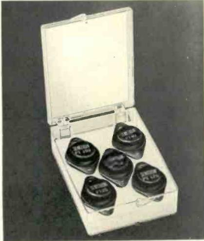
PNP power transistors and a complete replacement and interchangeability guide. Included are a high wattage transistor, medium wattage transistor, normal wattage transistor and a Semitron replacement for the 2N155 and the 2N176 types. More than 100 types may be replaced by Pack #5PT. Also, not shown, PT501 to replace all high wattage stud type power transistors. Semitronics Corp., 370 Broadway, New York 13, N. Y.
