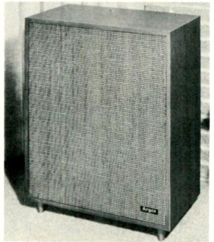
work to 8 ohm terminals on back. Cabinet uses tube-vented design to increase bass without booming, and boost effective power output. Covered with wood-grained pyroxylin in either walnut or blonde color; has cane grille and brass-finished legs. Internal volume, 3630 cu. inches. Size, 19¼"W, 22½"H, 10¼"D. \$39.95. Cabinet only, model AD-1A, \$24.95. Argos Products Co., Genoa, Ill.
