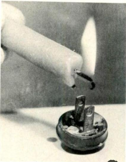
Loose connections and shorting plugs can be avoided by insulating a-c plug screw terminals with wax from a lighted candle after wires are attached.
