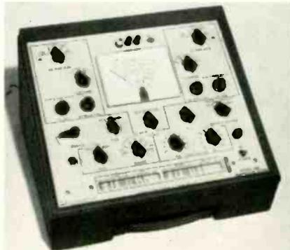
ranges cover from 0-0.5  $\mu$ a full scale to 0-25 ma full scale. A chopper and high-gain amplifier aid in leakage current measurement on the low-current
