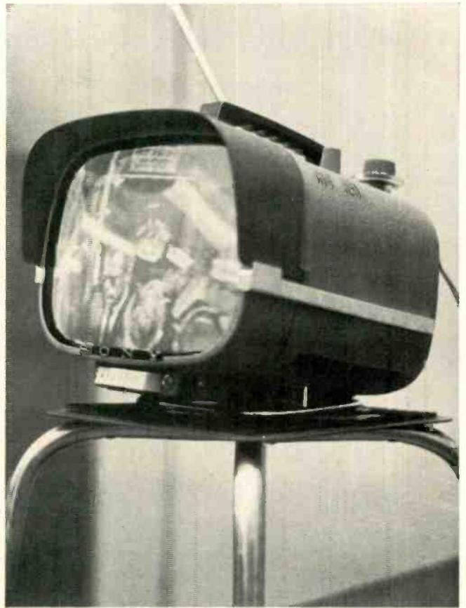
Sony's newest model portable TV weighs less than 14 pounds and only 17 pounds with battery pack. Its over-all dimensions are only 8½ x 7 x 9 inches.
