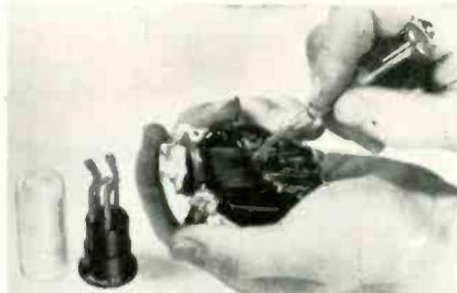
handle. Eight wrench sizes, fitting all sizes of tiny nuts found in electrical, automotive, aeronautical and other small mechanical devices, are available in two set-combinations as follows: 5/64, 3/32, 7/64, 1/8 and 5/32 in. in the first kit and 1/8, 5/32, 3/16, 1/4 and 5/16 in. in the second. All wrenches are heat-treated steel and use an interchangeable chuck-type handle. Moody Machine Products Co. Inc.
