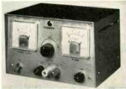
0-15 volts d-c at up to 3 amps. Designed for continuous duty, output is regulated to remain within .1% of indicated voltage with input varying from 105 to 125 volts. Filter circuitry is full wave, series shunt regulated, with 4 power transistors. Ripple factor is 10 mv RMS at 50% load, and 30 mv RMS at full load. All components are short circuit protected. Weight, 5 1/4 lbs. Size, 8 3/8 in. x 6 7/8 in. x 5 3/8 in. \$89.50. George Harmon Co., Inc.
