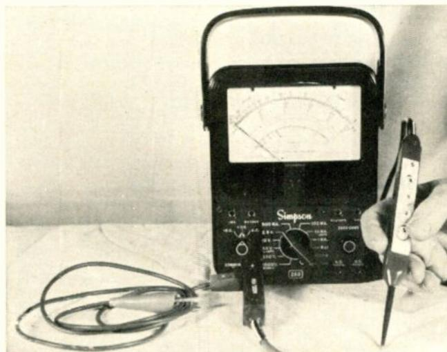
Speedprobe shown connected to meter. With the meter function switch set to 2.5 volts, the probe will measure voltages on scales equivalent to 2.5, 10, 150, 250, and 1000 volts by probe button selection.
