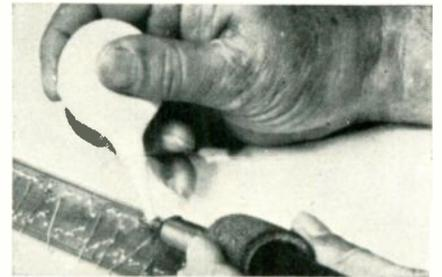
excess heat. Saves time and promotes neatness in solder work. Is effective in removing solder from hard-to-reach and otherwise inaccessible places. Solder pellets cool quickly inside the bulb. \$1.10. Macdonald & Company.
