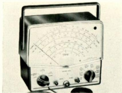
VTVM made by Triplet. Frequency response of this instrument can be extended to 250 mc with a special probe.
