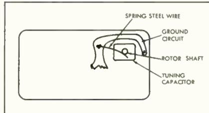
Noisy variable capacitors can be repaired by soldering a spring steel strip to PC board ground. Other end of spring is tensioned against rotor shaft.
