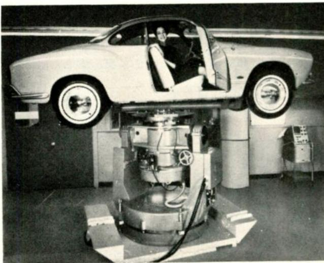
A 2000 lb sports car and its attractive passenger literally floats on air to demonstrate the load capacity of a precision air bearing servomotor turntable. A similar type, designed and built by Dunn Engineering Corp., will test the inertial guidance system of the Saturn rocket. The turntable rotor rests on a thin film of compressed air, instead of the conventional ball or roller bearings.
