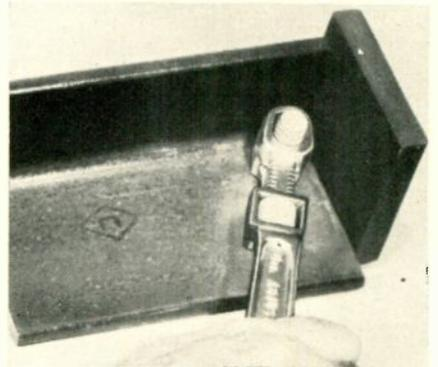
positive "four-sided jaw grip" on a hex nut or bolt head which it is said practically eliminates the possibility of rounding off or damaging the corners, and prevents slipping and injury to knuckles. \$3.98. Neff Enterprises, Inc.
