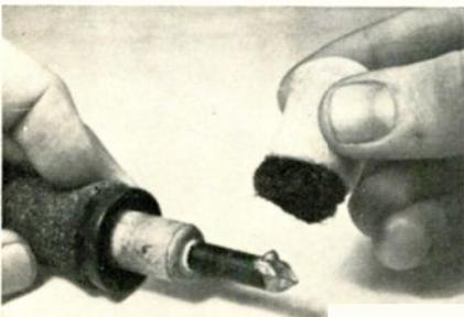
Steel wool used to clean soldering irons can be held in a rubber tip found on furniture legs.
