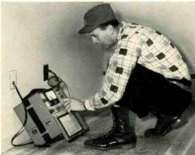
Technician uses Jerrold's Model 704B field strength meter to measure TV signal at a master distribution outlet.
