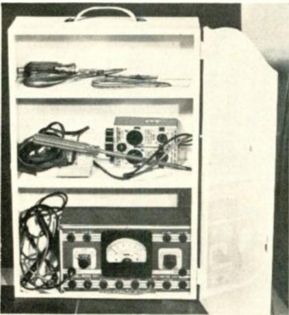
A handy bench mirror and tool cabinet can be made by attaching a handle to a standard medicine chest.
