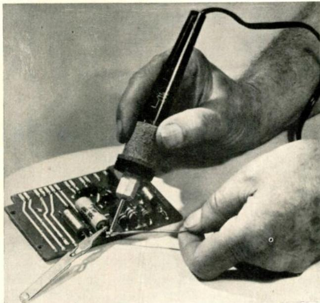
point. This is the time to make a more complete visual inspection. Resistors are seldom damaged in transistor radios since the power involved is limited. Don't wait till the last check, however, to test resistors—they do fail. Some manufacturers use low wattage resistors in low resistance emitter circuits which change value easily.
