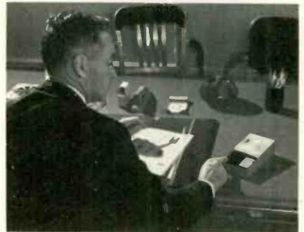
service in small offices, stores, shops, homes, and similar installations requiring a maximum of seven stations. Case is only 8x4x2 in. A six-position sliding switch selects other stations in the system. A thumb wheel adjusts the sound volume. Each master station is plugged into a standard 110 vac electric outlet. "Slave" stations do not require an outside power supply. General Dynamics Electronics.
