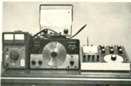
Instruments checked this month by ET editors were EICO's variable a-c supply, a Triplet VTVM, Heathkit's transistor tester and a Precision r-f signal generator. All are "tops" in their category.
