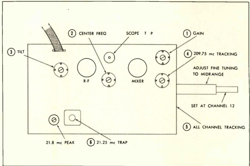
have such a test point, connect the scope's vertical input to the center of the grid network on the mixer stage. In either case, use a 10K resistor in series with the scope lead. Keep the generator and marker inputs as low as possible. Excessive signal injection tends to distort the response curve.
