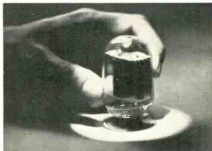
compactron type 6GE5 is 2.5 in. which is 1 3/16 in. shorter than the seated height of its conventional-tube counterpart, the 6DQ6B, or a reduction of 32.5 per cent in space requirement for the horizontal deflection amplifier. General Electric.
