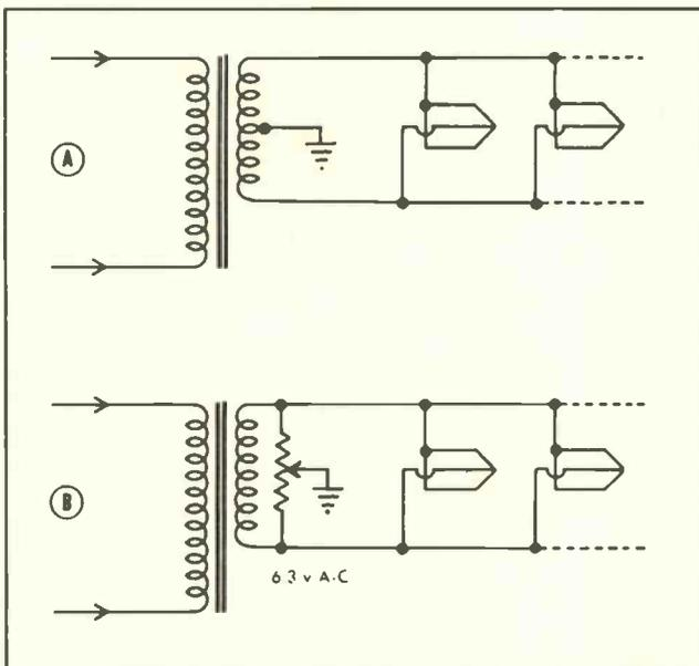
Fig. 2 (A)—Standard method of minimizing hum in low level heater circuits. (B)—A transformer without a center tap can be effectively center tapped with a potentiometer. This method has the advantage of being adjustable for a more precise balance.
