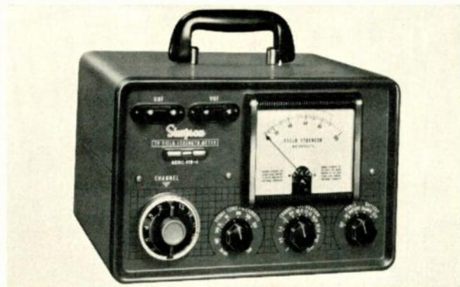
Simpson's Model 498A calibrated field strength meter can be operated on 117 vac or on batteries.
