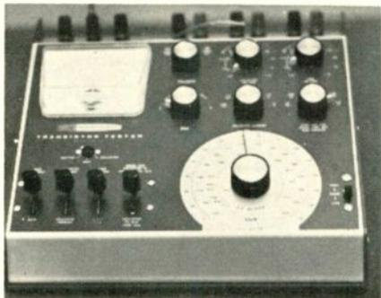
Transistor tester by Heathkit checks all major transistor parameters.
