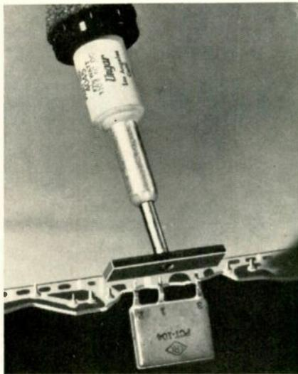
Ungar's bar-type desoldering tip may be employed for easy removal of multiple inline-terminated components.
