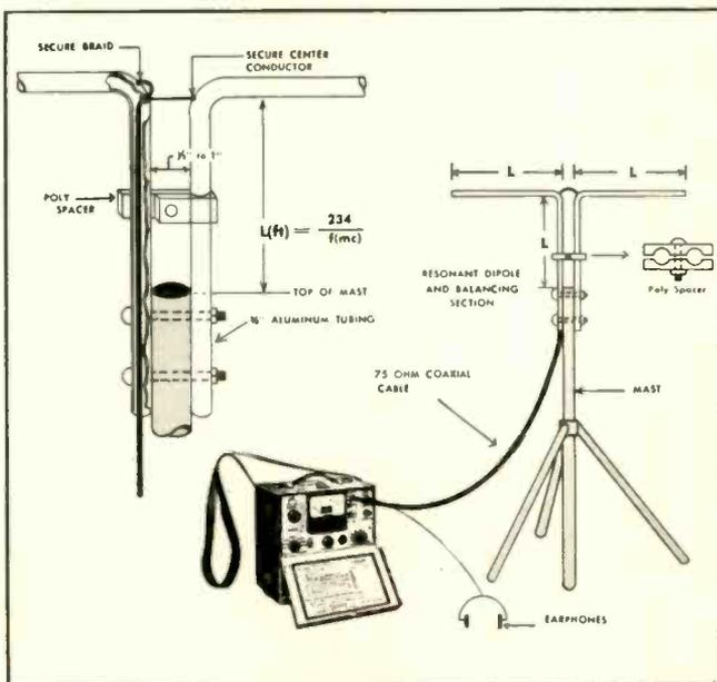
Fig. 1 — Specifications for dipole antenna used with field strength meter for intensity surveys and for RFI interference location. It can be altered for vehicular mounting.
