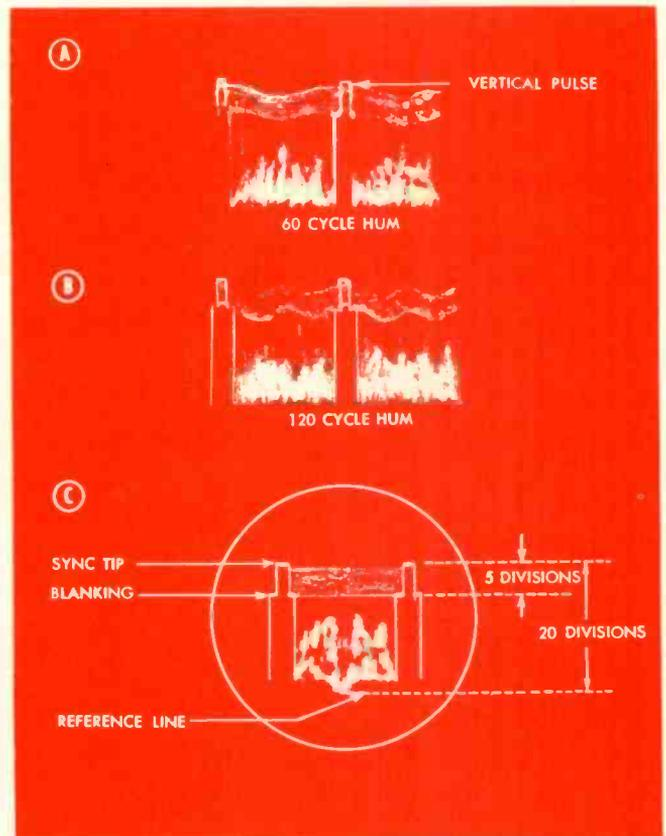
Fig. 2 (A)—60 cps hum on composite video signal as it appears on scope when d-c coupled from field strength meter. (B)—120 cps hum. (C)—Percentage of sync pulse height can easily be compared with total composite video amplitude.
