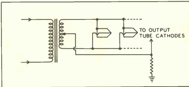
Fig. 1—Coupling of a-c between the filaments and cathodes of low level stages is greatly reduced by elevating the filaments with a positive d-c voltage. Often the d-c is supplied by the cathode voltage on the output tubes.
