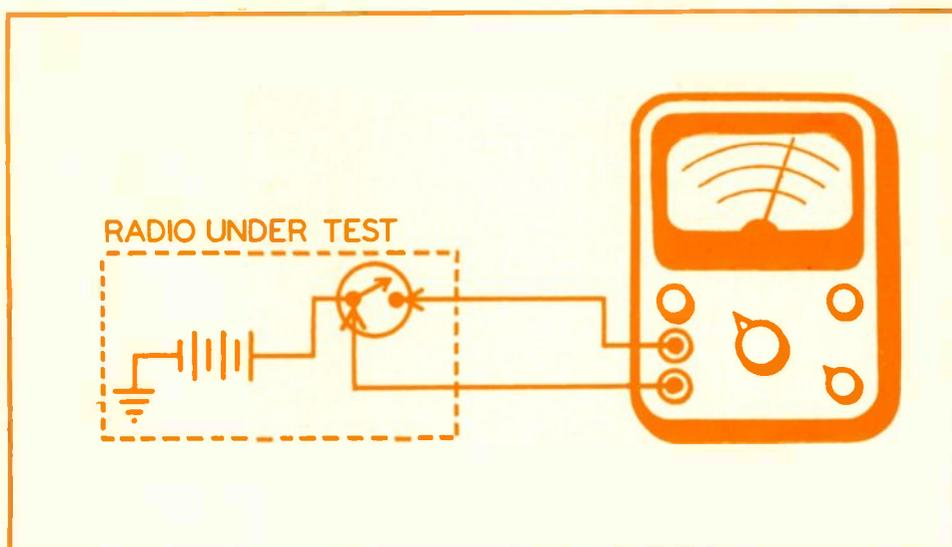
Current drain can be measured without breaking battery connections by inserting a milliammeter across the on-off switch with the set turned off.
