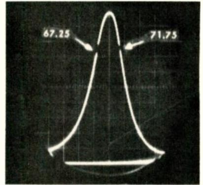
Typical r-f response taken from a properly aligned tuner on channel four. Note the symmetry of the waveform.
