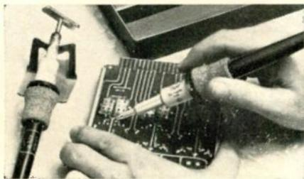
Low wattage iron equipped with slotted desoldering tip may be used to remove capacitor from printed circuit board. Iron at left is equipped with bar type desoldering tip.
