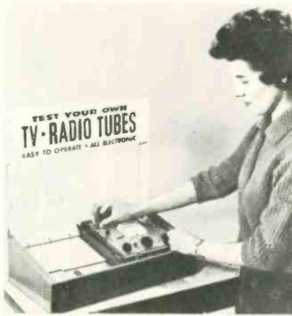
two stage d-c amplifier, selenium rectifier power supply, single 5 ma meter which indicates results for both grid circuit and tube merit tests. \$79.50 with self-service display. Seco Electronics, Inc.
