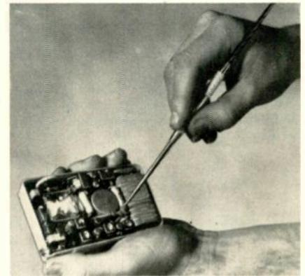
Moody's HPS-2 hooked point scriber is another aid in checking transistorized circuit connections and general probing.
