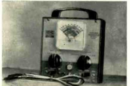
tures include a wide angle meter, three tests (shorts-leakage-gain), transistor socket for "out-of-circuit" testing and zero adjustments on meter. G C Electronics Co.
