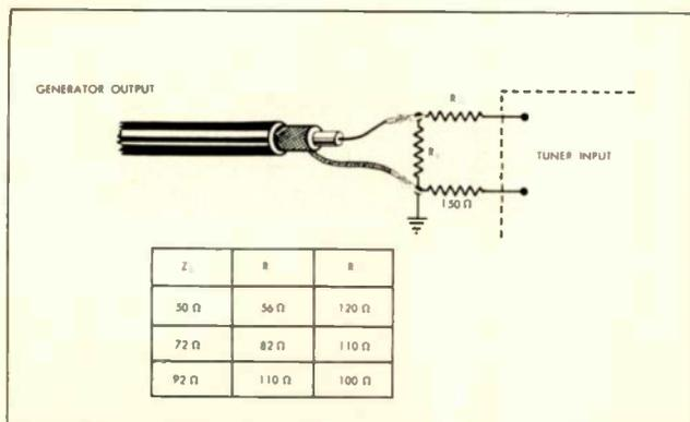
Fig. 1 — Network to terminate sweep generator output to 300 ohm input at the tuner.  $Z_0$  is equal to the generator impedance. The inset chart shows network values for three common generator impedances.
