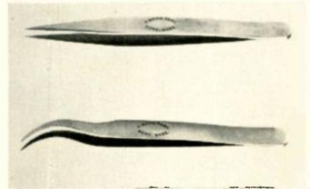
Mark Tool's straight and curved point tweezers can serve as needle nose plier on midget type transistorized radios.
