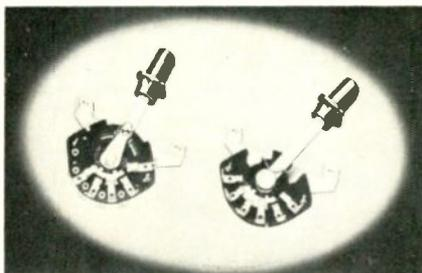
these switches are available as single units or as ganged assemblies with end brackets for mounting. Rated at 1.5 amp at 28 vdc, 230 ma at 115 vac, with a current carrying capacity of 9 amp. Clips and rotor contacts are silver plated brass and the clips will accommodate up to #18 wire. Silver alloy clips are also available. Insulation is laminated phenolic with a voltage breakdown of 1000 v rms. Centralab.
