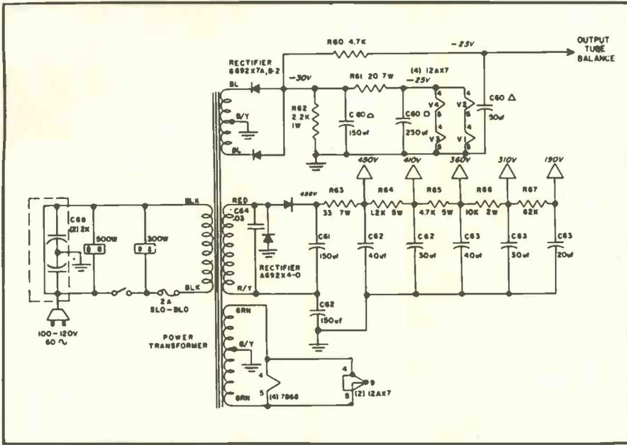
Power supply used in a Sherwood amplifier uses d-c to supply filament voltage for low level stages. Heavy filtering is used for both B+ and filament voltages. A small d-c voltage is also used in a balance circuit for the output tubes.
