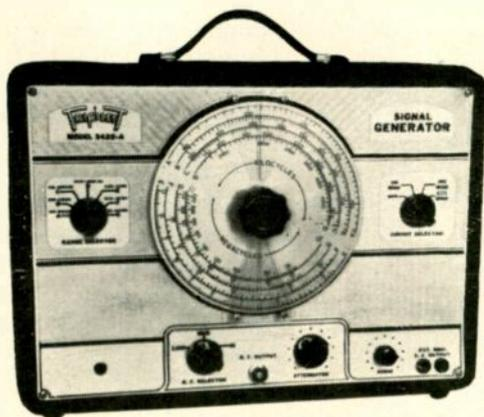
*Triplet Model 3432-A signal generator, at \$119.50. — A signal generator is basically a very simple piece of equipment. At the most, it seldom has more than three tubes and more frequently only two. Simplicity in most equipment is a difficult-to-achieve virtue — the 3432-A is simple.*
