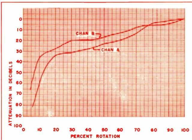
Fig. 1—Unmatched controls plotted to show variation of resistance.
