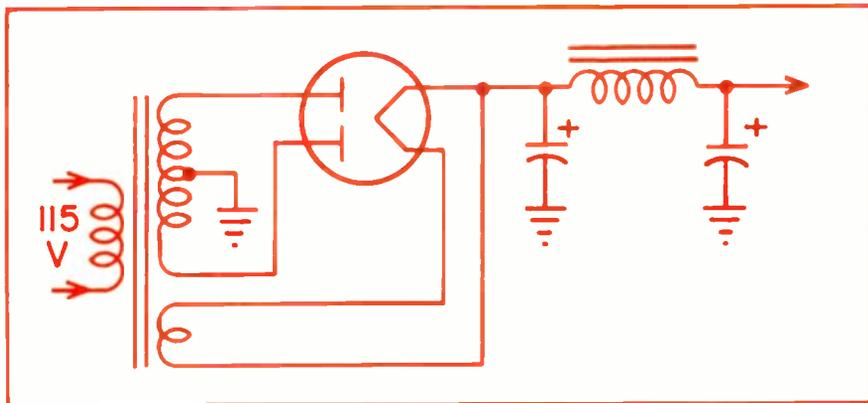
Fig. 3—Full wave rectifier circuit most frequently found in transformer powered sets.
