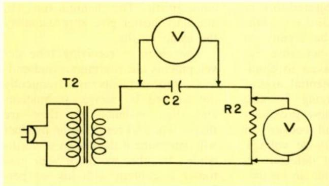
Fig. 2—Circuit arrangement for determining value of an unknown capacitance.
