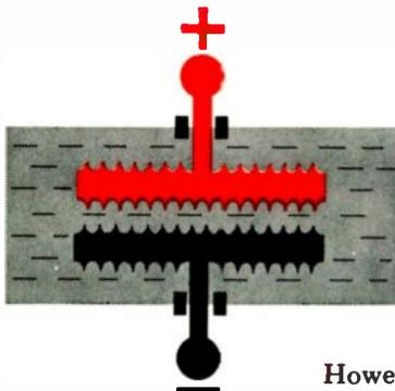
Aluminum electrolytic capacitors are widely used as filters in DC Power Supplies. This is because of their large capacitance in relatively small size. All in all, they do an efficient job of reducing ripple (hum) to acceptable levels.
