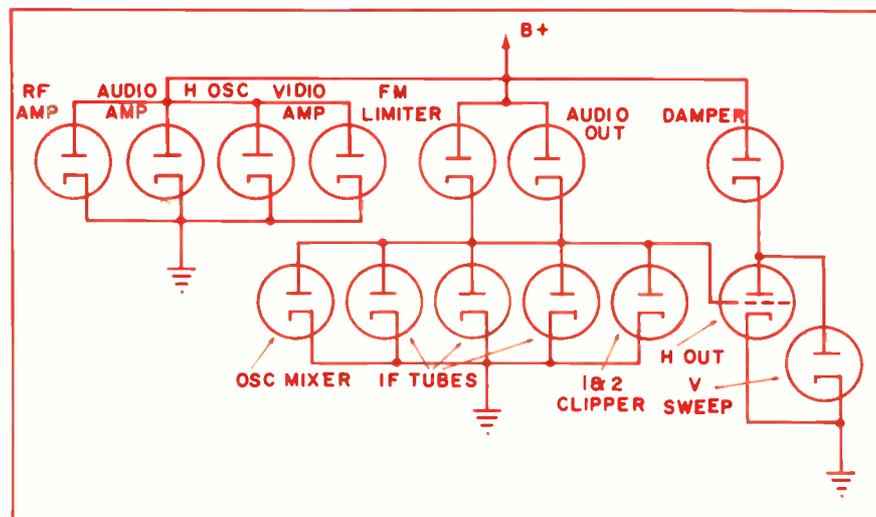
Fig. 2—Series parallel distribution of B+ to provide proper voltage to each stage. Malfunction in any stage can cause B+ variation.
