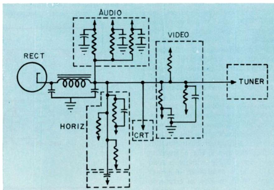
Fig. 1—Distribution of B+ in a typical TV receiver.
