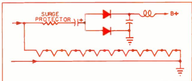
Fig. 5—Voltage Doubler Circuit used in many transformerless TV sets.
