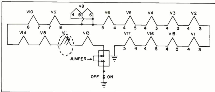
Ohmmeter check at the center of a series string eliminates half of the string from suspicion.
