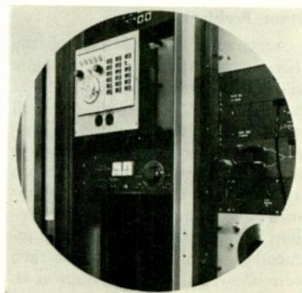
Rack-mounted FM broadcast monitor tuner used in Telstar tests.
