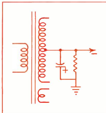
Fig. 4—A resistor in the ground return of a power transformer is sometimes used to develop a small negative voltage.
