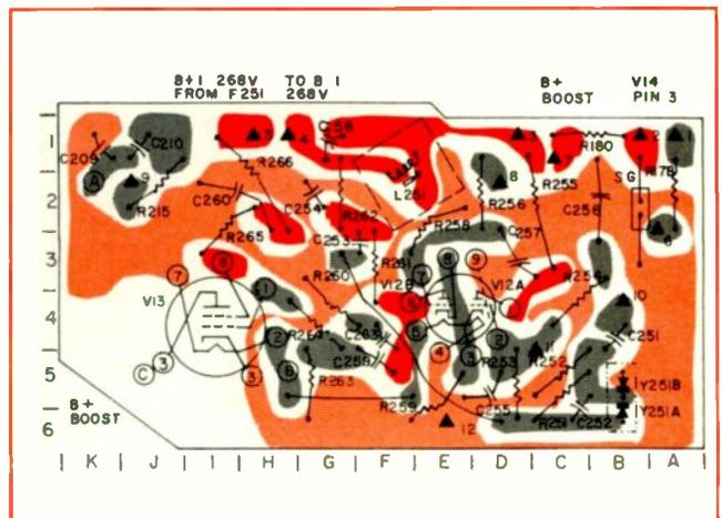
A small portion of a card contained in the colorgram package. The color scheme found on the schematic is carried on the PC card and throughout each set.
