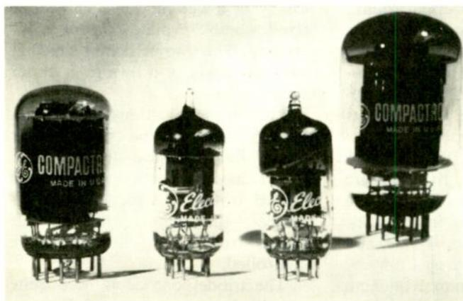
G-E compactron-type tubes for low power communications transmitters allows compact 2-way mobile equipment design.
