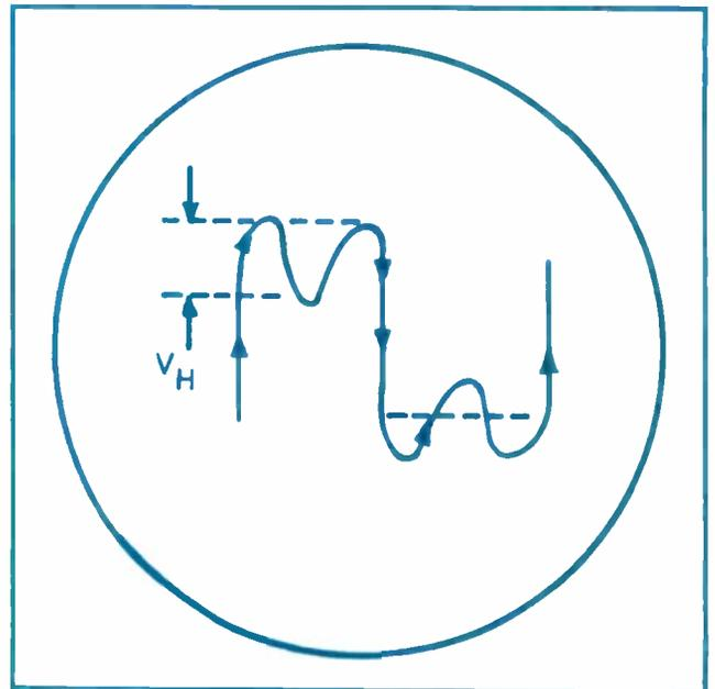
Fig. 2 — Appearance of a ringing square wave. A different number of cycles appear each time LC is tuned through a harmonic frequency of the square wave.  $V_h$  is the voltage of the harmonic.
