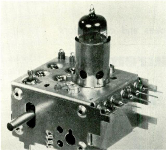
Waller Corporation FM tuner front end uses high-mu twin triode 12DT8, 6DT8 or 6AQ8.
