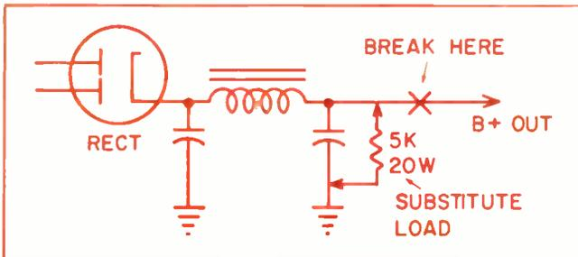
Fig. 6—Isolating a problem to the power supply or other circuits in a TV is best accomplished by disconnecting the supply and loading it with a suitable resistor.
