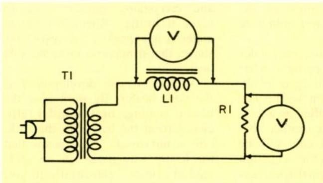
Fig. 1—Schematic of components connected in series for determining choke inductance.
