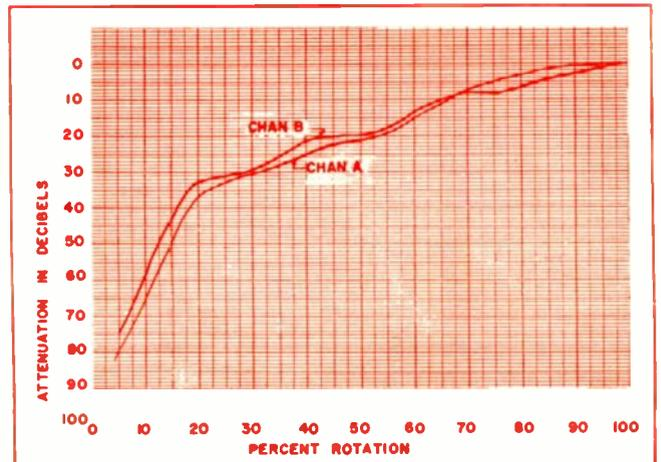
Fig. 2—Matched controls maintain less than 6 db deviation. Courtesy of CTS.
