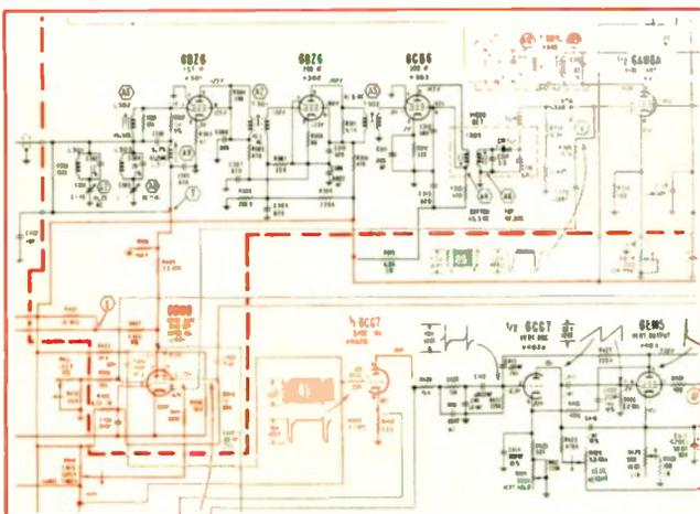
A portion of a typical schematic used in Colorgrams. As many as seven colors may be used on a single schematic to show the various sections of a receiver.
