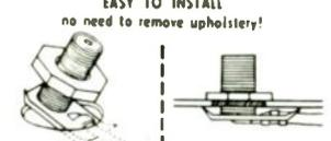
Mounts from outside by insertion through 3/8" hole. | Mounts flat; inside uses 3/8" hole.
