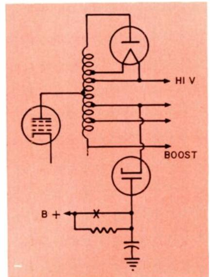
Premature failure and poor operation can often be blamed on too much B+. This voltage can be reduced by inserting 100 $\Omega$  of resistance in the damper tube's plate circuit, for every 10 v of excessive B+. The resistor should then be bypassed with a suitable capacitor.
