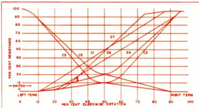
Fig. 3 — Curves for tapers commonly used by technicians: Linear, semi-log, right-hand semi-log, modified log with 20% center, right hand modified log with 20% center, modified log with 40% center and symmetrical-straight line. Courtesy of Centralab.
