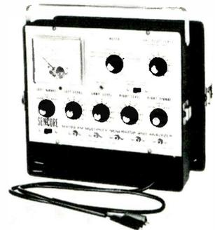
the FM stereo station under crystal controlled conditions. A built-in meter, calibrated in db and P-P v, enables the user to set the left and right channels and 19 kc
