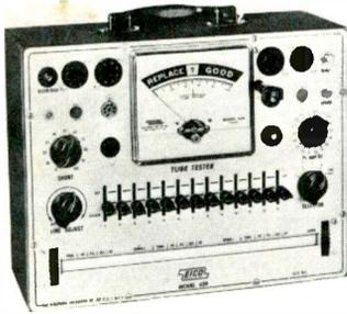
and continuity. A 4½-in. meter has a 3-color REPLACE-WEAK-GOOD scale and 0 to 100 scale for matching. Tests 7- 9- and 10-pin miniatures, octal, loctal, 5- and 7-pin nuvistors, novars and compactrons. Types tested include series string, magic eye, VRs. Adapter available for testing all CRTs, both color and B/W. EICO
