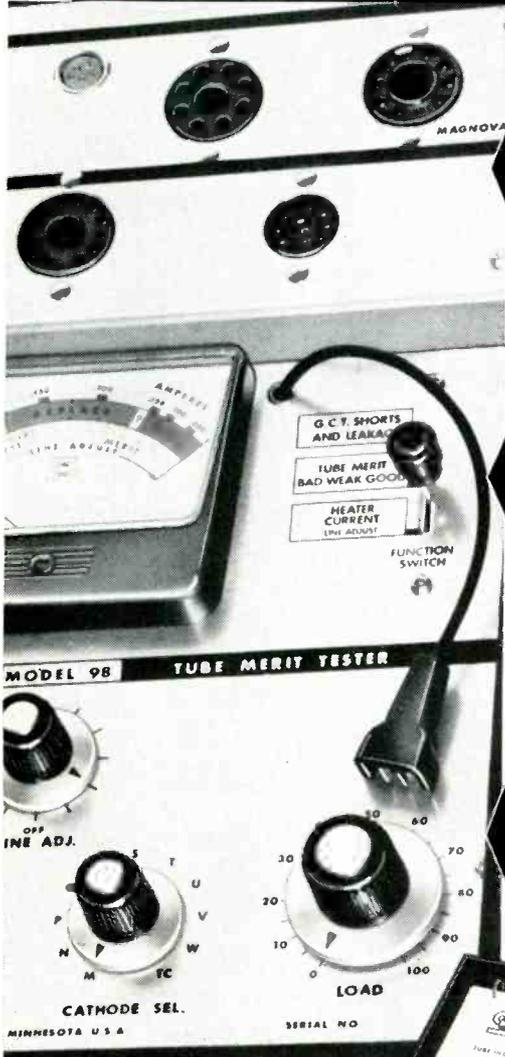
**A SECO PLUS!** Replaceable socket chassis plugs into metering chassis. Can be economically replaced as it wears out or becomes obsolete. Available with special sockets upon request. Guaranteed up-to-date for all modern receiving tubes including novars, novistors, 10-pin types, compactrons and MAGNOVALS.
