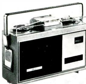
recorder, model 101, is announced. It weighs 7 lb and uses "D" type flashlight batteries. Frequency response is 80-8000 cps, it is said. It can record from a radio, phonograph, or TV as well as the microphone by using a special input jack. The unit operates at 1 7/8 in./sec and will provide up to two hours playing time on a single 4-in. reel, according to the maker. The recorder measures 11 x 3 3/4 x 8 in. North American Philips.
