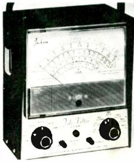
times more sensitive than conventional movements, it was reported. Specifications: 6 in. meter face; ac accuracy 5% of full scale; dc accuracy 3% of full scale; frequency 20 cps to 3 Mc; input resistance 10 MΩ. Ranges dc 0 - 1 - 5 - 10 - 100 - 500 - 1000; RMS 0 - 1 - 5 - 10 - 50 - 100 - 500 - 1000; P - P 0 - 2.8 - 14 - 28 - 140 - 1400 - 2800. Jackson.
