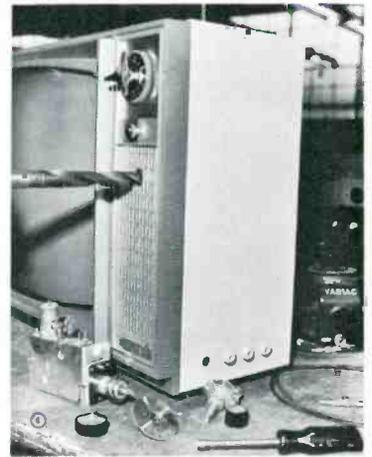
■ A UHF television converter kit that can be installed in about 45 minutes in consoles, table models, and most portables, has been developed. The converter tuner permits the TV dealer or service technician to customize television sets for his customers, make VHF television trade-ins more saleable, or replace defective UHF tuners. It tunes all channels, 14 through 83. The kit contains all necessary parts including tuner.
