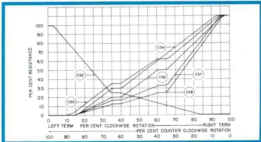
Fig. 4—Special tapped resistance tapers. C52: RH taper; C54: LH linear taper; C55: LH linear taper; C56: LH taper; C57: LH taper; C58: LH taper.
