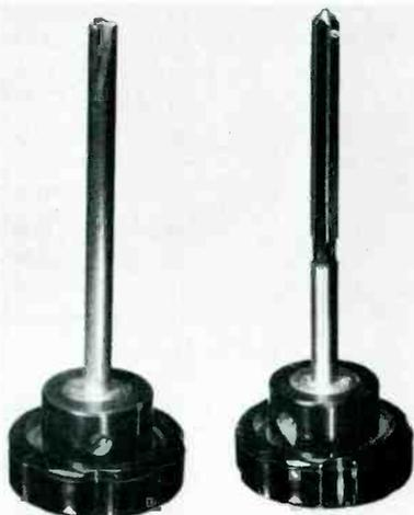
Knob reamers with handles made from old instrument knobs. At left is "home made" reamer; at right is commercially made fluted reamer.
