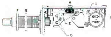
Top view of converter shows terminals used in hookup.
