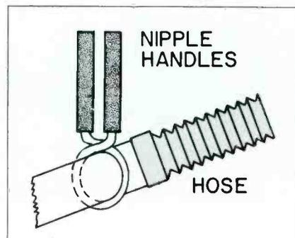
Pipe nipples serve as handles for clamp removal.
