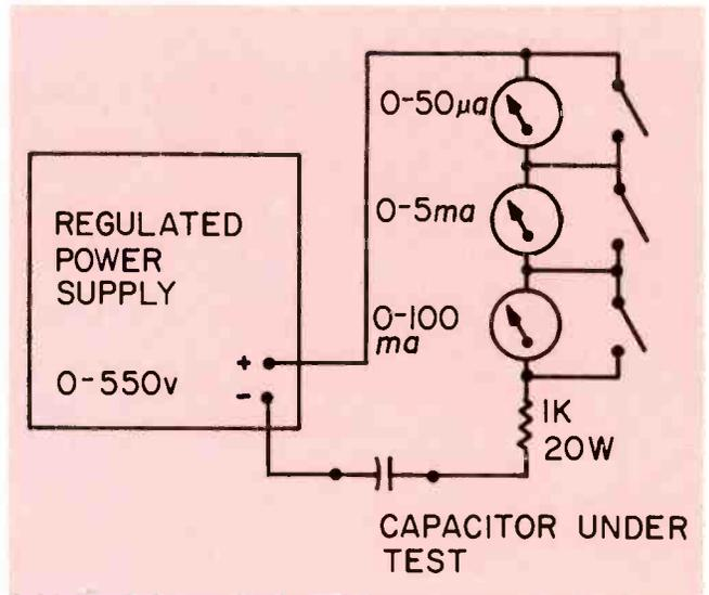
Fig. 1—Basic circuit used to measure electrolytic capacitor leakage current.
