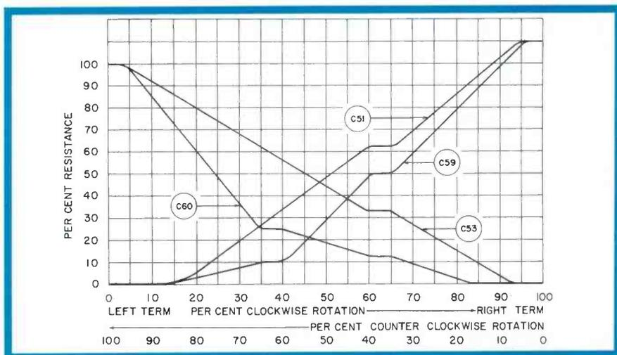
Fig. 3—Special tapped resistance tapers. C51: LH linear; C53: RH linear; C59 LH semi-log; C60: RH semi-log.
