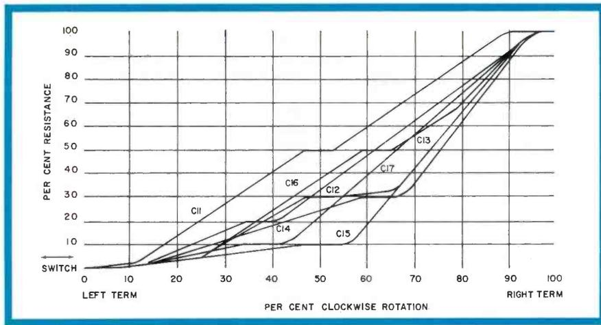
Fig. 2—Standard tapped resistance curves. C11: taper tapped, tone control or in TV or vert. and hor. centering. C12, C13, C14, C15, C16 and C17: used as vol. control with tone compensating tap.
