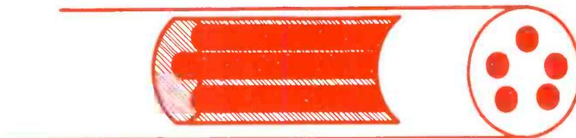
Fig. 2 — Cut-a-way sketch of a 5-core solder.
