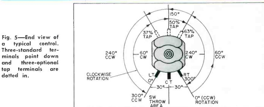
Fig. 5—End view of a typical control. Three-standard terminals point down and three-optional tap terminals are dotted in.
