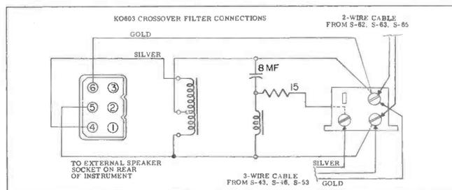
Magnavox connections for two types of speaker units when used with KO603 kit in conjunction with Astro-Sonic 100-w models.
