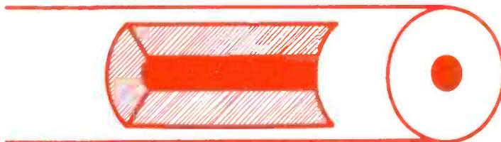
Fig. 1 — A cut-a-way sketch of single-cored solder.
