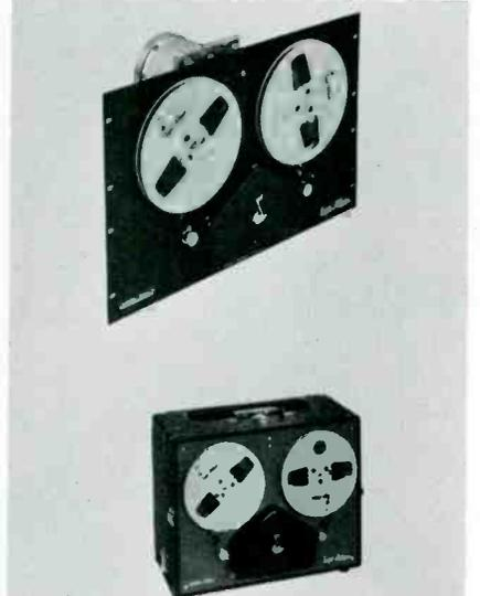
the player will accept programs of any duration from 20 sec to 8 hours, recorded on a suitable 1/2 track recorder at speeds of 1-7/8, 3-3/4, or 7-1/2 ips. A program can be started by an external momentary pulse of 6 to 12 v ac/dc to the player via a built-in connector; the entire program is then played to the end of the recording, the tape reverses and immediately shuts off, waiting for the next "start" pulse, specifications indicated. Tape-Athon.
