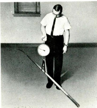
A fiberglass encased antenna, weighing eight pounds, is developed for two-way radio base stations operating in the 25 to 50 Mc range. It is said the antenna was designed to improve message reception and transmission by minimizing static
