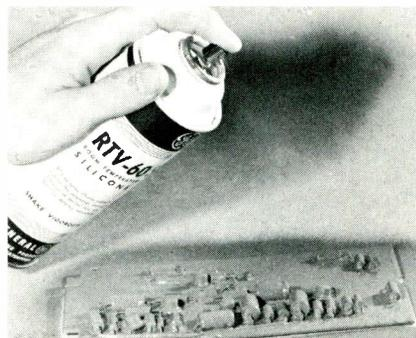
Liquid rubbers permit encapsulation of circuitry by the spray method.
