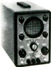
**EICO 430 PORTABLE GENERAL PURPOSE 3" SCOPE** Remarkably fine compact scope. Excellent for servicing audio, communications, and industrial equipment. Ideal as a ham shack monitor. Flat-face 3" CRT with mu metal shield eliminates affects of external fields. Vert. amp. flat from 2 cps to 500 kc, —6 db at 1 mc; 25 mv rms/cm sensitivity. Horiz. amp. from 2 cps to 350 kc, 0.25 v rms/cm sensitivity. Sweeps from 10 cps to 100 kc. Kit \$69.95; Wired \$99.95.
