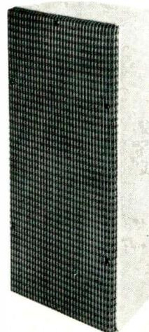
compact, rugged, metal enclosure that is fully lined with Tuflex insulation and ported for optimum low-frequency response, the announcement said. Power, 15 w; impedance, 8 Ω; response, 70-15,000 cps. Size 18 x 8 x 5½ in. Atlas Sound.
