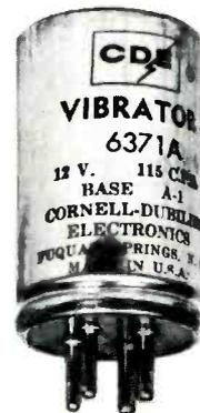
include a contact arrangement utilizing the combined advantages of tungsten "button" contacts and Molybdenum leaf contact members, improved magnetic circuit and driving coil, and reduced overall length to 2 $\frac{5}{8}$  in. excluding the pin base. Available for 6 and 12 v equipment. Rated for continuous duty at 6 and 4 amp respectively. Cornell-Dubilier.
